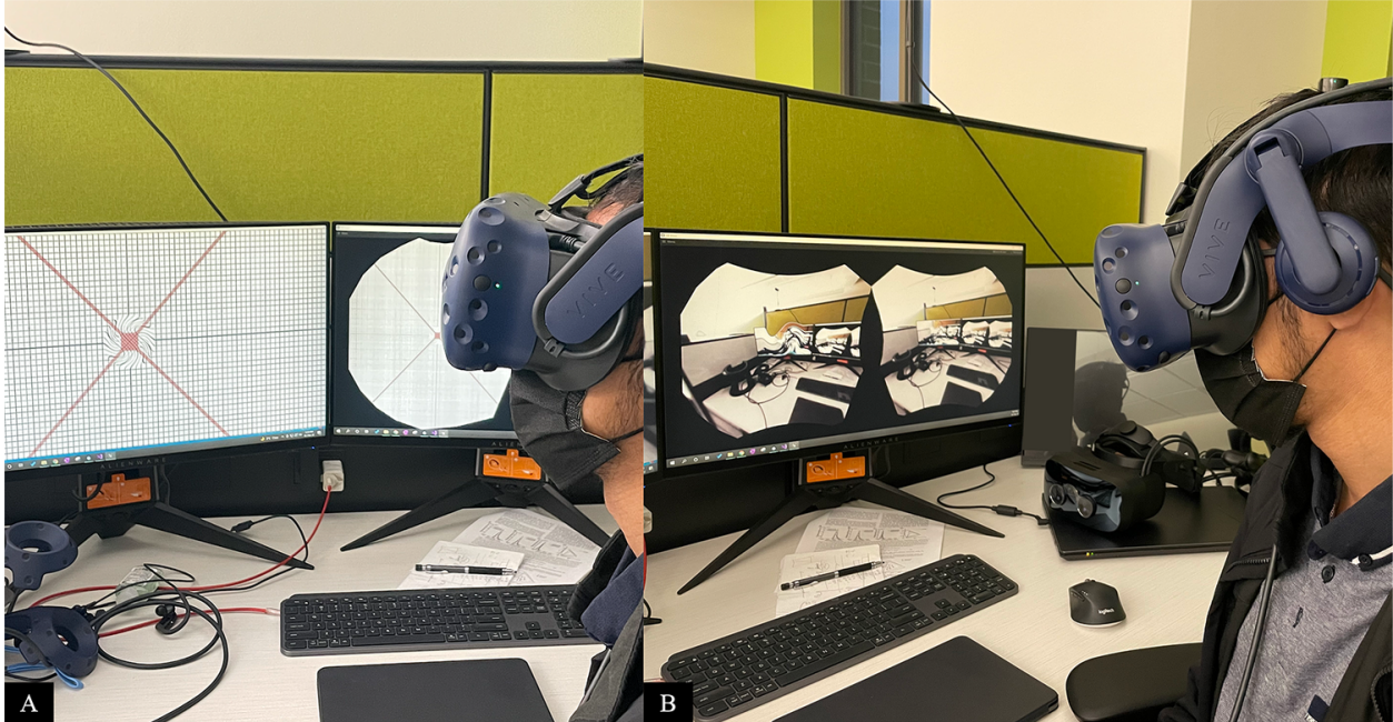
Figure 6.1: Simulated metamorphopsia on an Amsler Grid (a) and through the augmented reality camera feed
