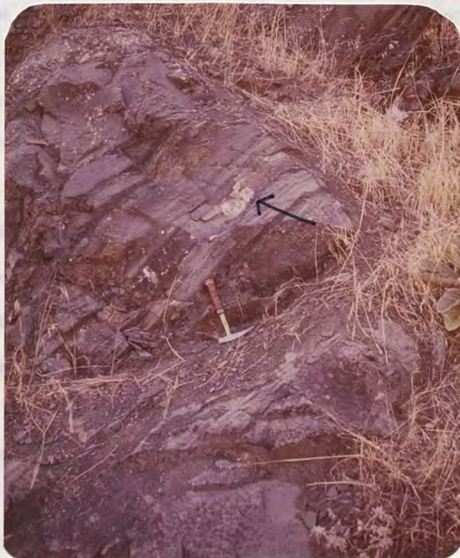
Figure 8. - Limestone lens in thin-bedded shales and graywacke, on the western side of Stony Creek.
