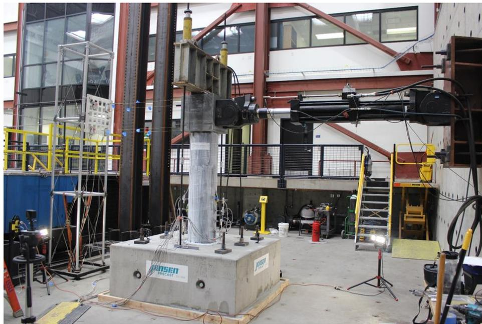
Figure 4-6. Overall test setup of UHPC columns under combined axial and lateral loading
