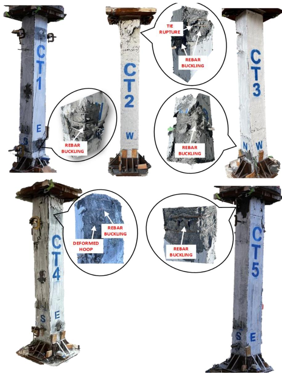
**Figure 3-15.** Damage patterns for all five UHPC columns after axial failure
