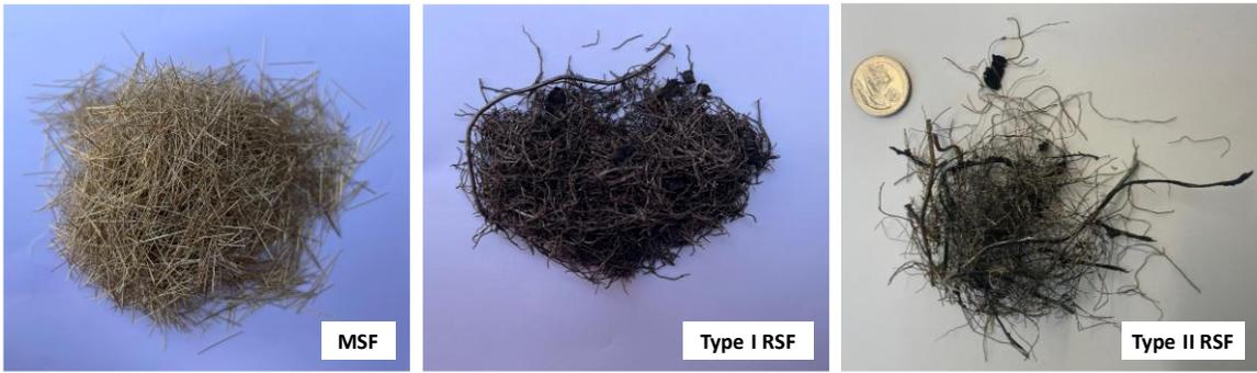
**Figure 2-1.** Samples of MSF, Type I RSF, and Type II RSF
