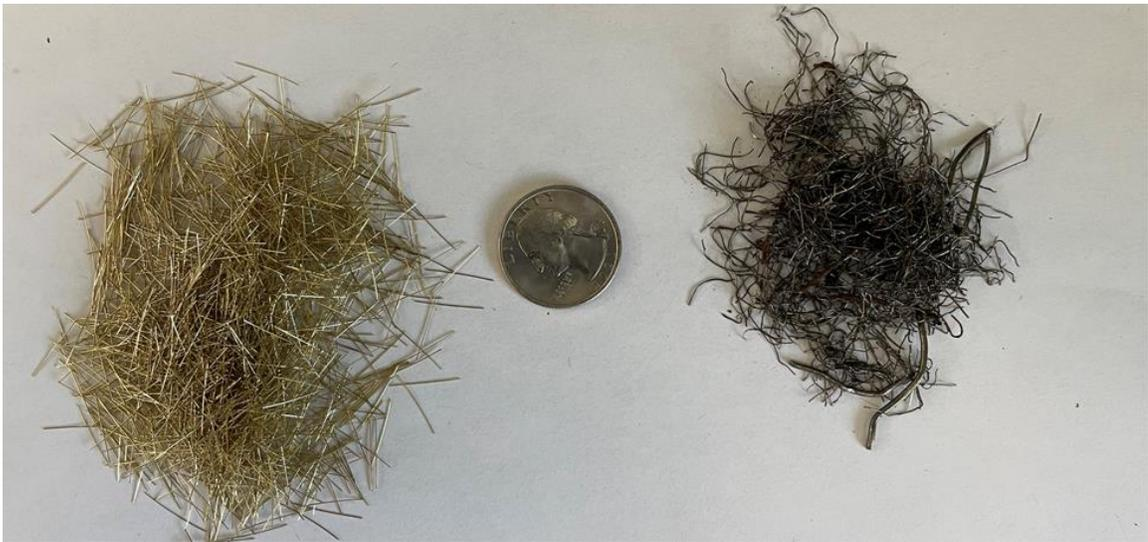
Figure 3-3. Comparative appearance between the MSF and RSF used in this study
