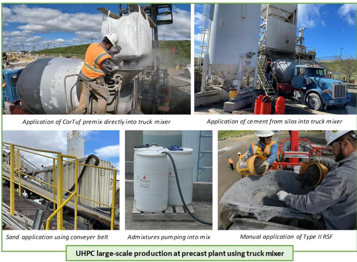
**Figure 2-3.** Photographs of the different UHPC constituents and high-shear versus truck mixing procedure
