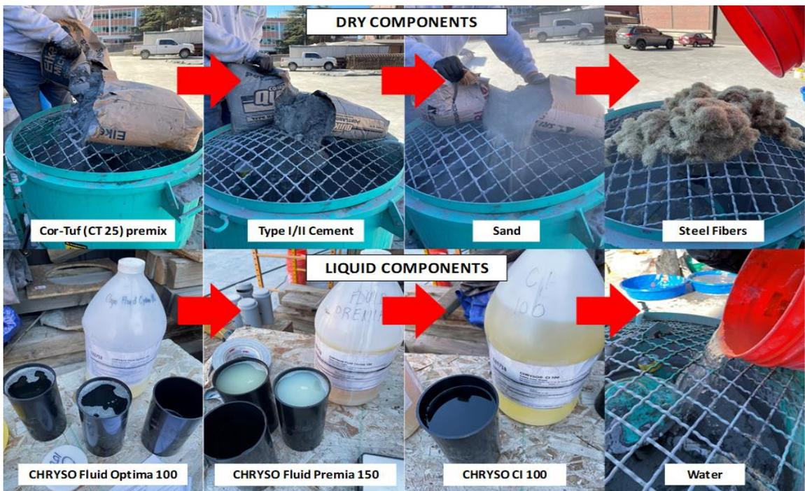
Figure 3-4. UHPC material batch sequencing using a high-shear mixer
