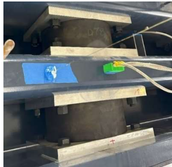
Figure 25: Stringpots attached to the soil box
