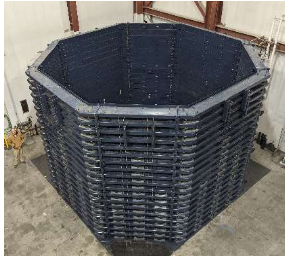
Figure 5: Picture of the assembled soil box in the laboratory
