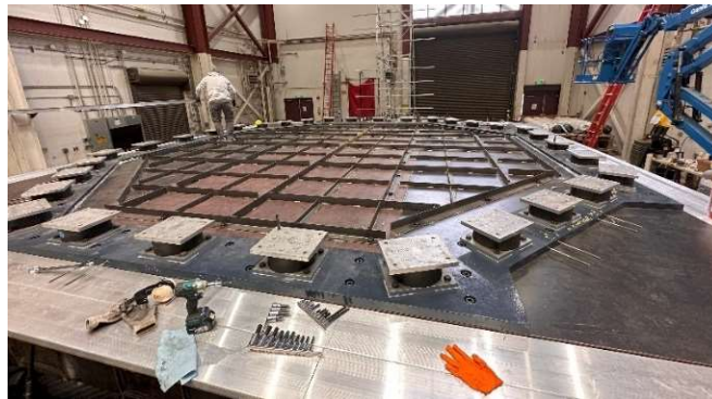
Figure 9: Soil box base platform attached to shake table
