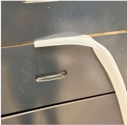
Figure 12: Silicone tube sealing the gap
