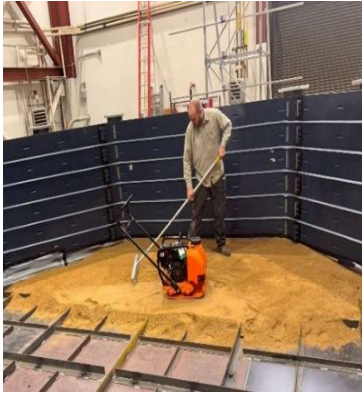
Figure 20: Leveling the soil
