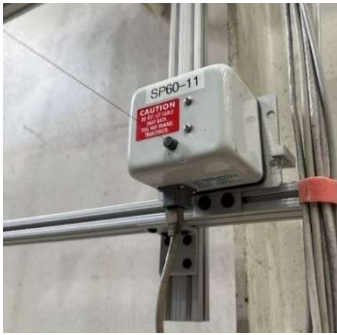
Figure 24: Stringpot fixed to the stationary surface
