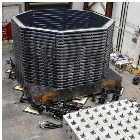
Figure 1: Soil box built at the University of Nevada, Reno
