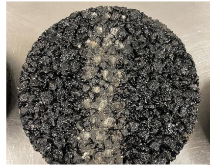
Figure 60. Lockwood Tested Sample under Studded Tire Top View (Condition 3)
