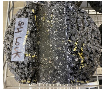
Figure 45. Lockwood Tested Sample under Non Studded Tire Top View (Condition 2)
