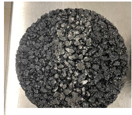
Figure 57. Mustang Q&D Tested Sample under Non-Studded Tire Top View (Condition 3)
