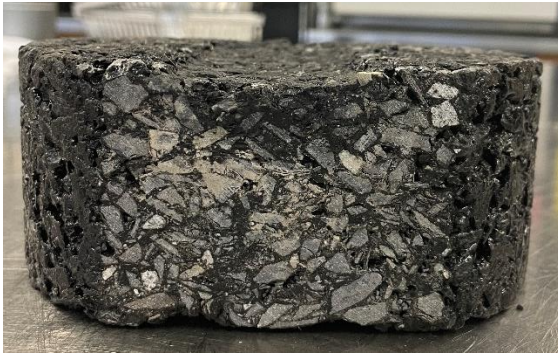
Figure 50. Mustang Western Nevada Tested Sample under Studded Tire Side View (Condition 2)
