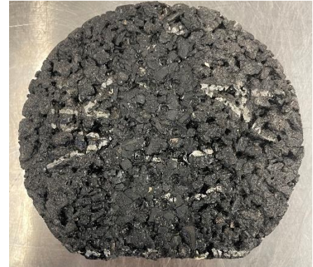
Figure 51. Mustang Western Nevada Tested Sample under Studded Tire Side View (Condition 2)
