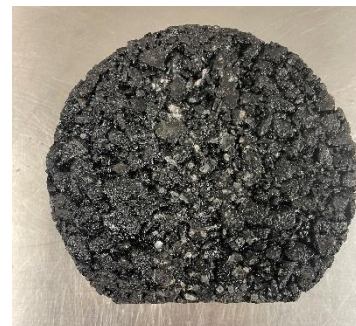
Figure 69. Mustang Western Nevada Tested Sample under Studded Tire Top View (Condition 3)
