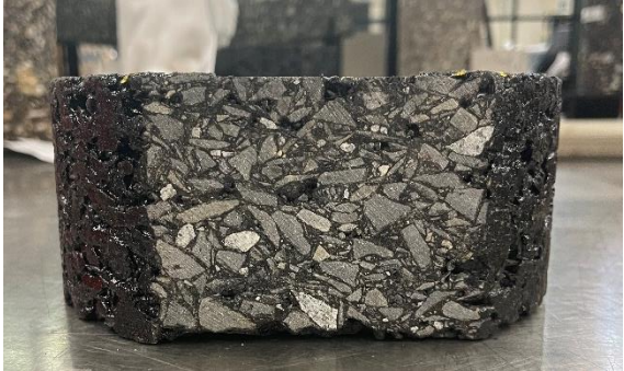
Figure 30. Mustang Western Nevada Tested Sample under Studded Tire Side View (Condition 1)
