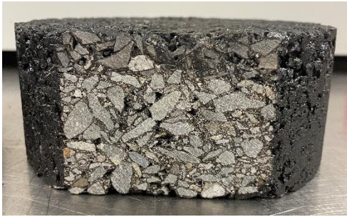
Figure 67. Mustang Western Nevada Tested Sample under Studded Tire Side View (Condition 3)
