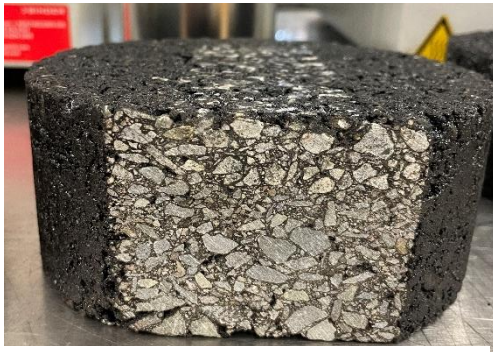
Figure 66. Spanish Springs Tested Sample under Non Studded Tire Side View (Condition 3)
