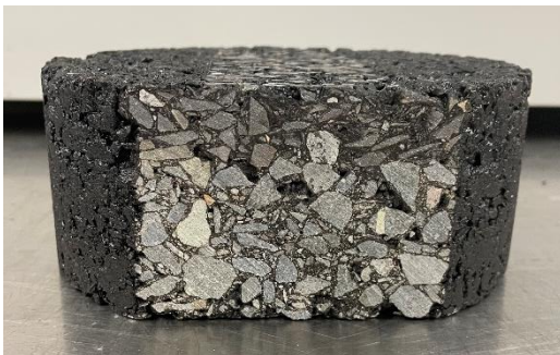
Figure 70. Mustang Western Nevada Tested Sample under Non Studded Tire Side View (Condition 3)
