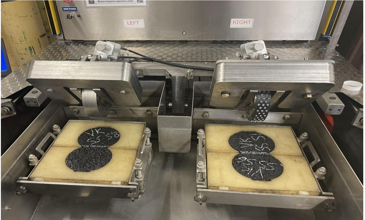
Figure 8. Hamburg Wheel Track Test Setup
