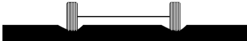
Figure 2. HMA Raveling due to Studded Tires (WSDOT, 2008)
