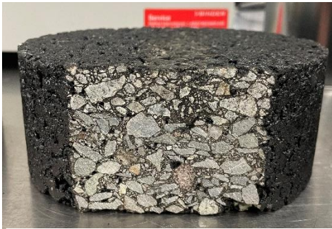
Figure 64. Spanish Springs Tested Sample under Studded Tire Side View (Condition 3)
