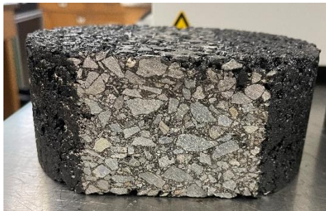
Figure 58. Mustang Q&D Tested Sample under Non-Studded Tire Side View (Condition 3)
