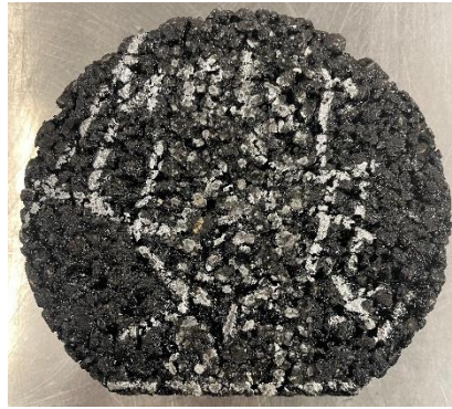
Figure 35. Brunswick Tested Sample under Studded Tire Top View (Condition 1)
