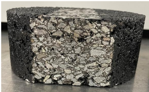
Figure 61. Lockwood Tested Sample under Non Studded Tire Side View (Condition 3)
