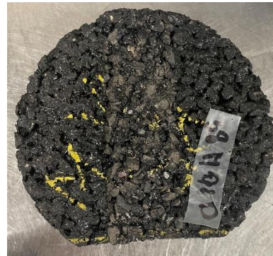
Figure 38. Mustang Q&D Tested Sample under Studded Tire Top View (Condition 2)
