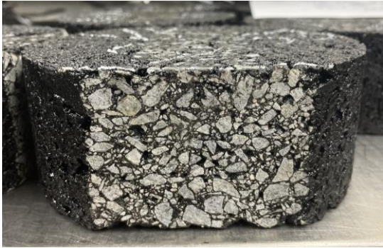
Figure 28. Spanish Springs Tested Sample under Non Studded Tire Side View (Condition 1)
