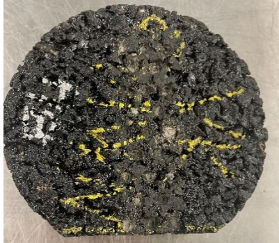
Figure 29. Mustang Western Nevada Tested Sample under Studded Tire Top View (Condition 1)
