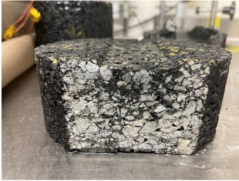
Figure 46. Spanish Springs Tested Sample under Non Studded Tire Side View (Condition 2)
