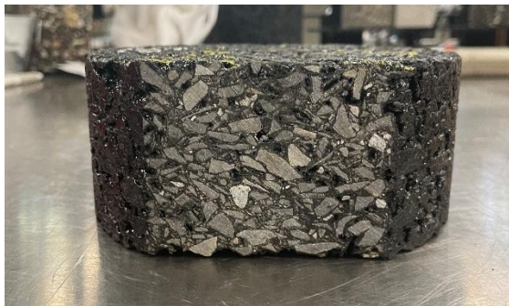
Figure 32. Mustang Western Nevada Tested Sample under Non Studded Tire Side View (Condition 1)
