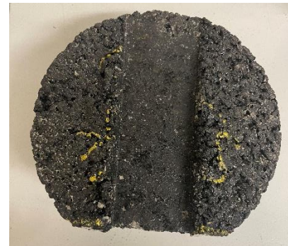
Figure 49. Spanish Springs Tested Sample under Non Studded Tire Side View (Condition 2)
