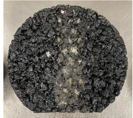
Figure 56. Mustang Q&D Tested Sample under Studded Tire Top View (Condition 3)
