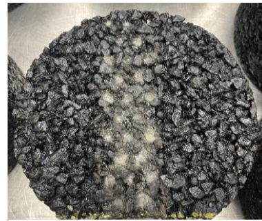
Figure 21. Lockwood Tested Sample under Studded Tire Top View (Condition 1)
