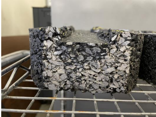
Figure 41. Mustang Q&D Tested Sample under Non Studded Tire Side View (Condition 2)
