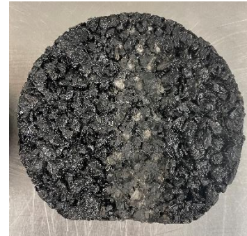
Figure 68. Mustang Western Nevada Tested Sample under Studded Tire Side View (Condition 3)
