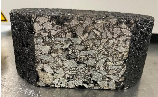
Figure 55. Mustang Q&D Tested Sample under Studded Tire Top View (Condition 3)
