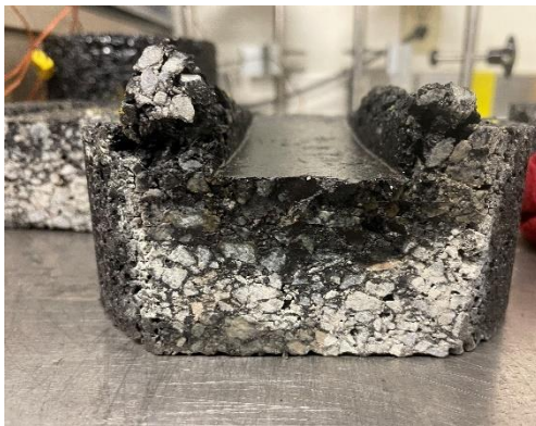
Figure 48. Spanish Springs Tested Sample under Non Studded Tire Side View (Condition 2)
