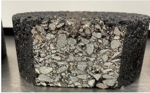
Figure 59. Lockwood Tested Sample under Studded Tire Side View (Condition 3)
