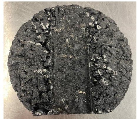
Figure 53. Mustang Western Nevada Tested Sample under Non Studded Tire Top View (Condition 2)
