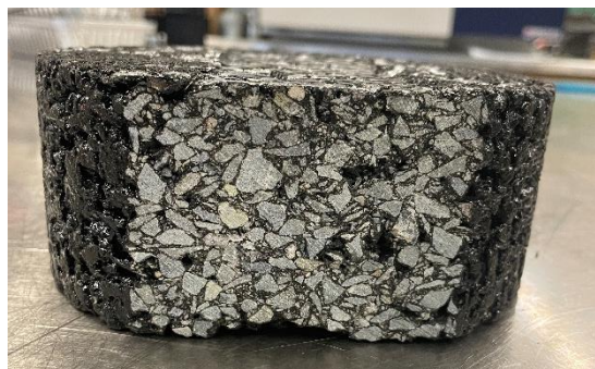
Figure 34. Brunswick Tested Sample under Studded Tire Side View (Condition 1)
