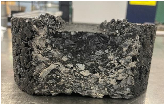
Figure 52. Mustang Western Nevada Tested Sample under Non Studded Tire Side View (Condition 2)
