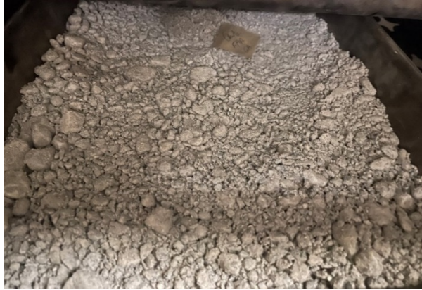
Figure 8. Fully Coated Aggregates with Cement
