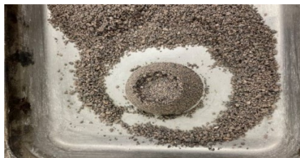
Figure 7. Checking for SSD Condition in the Fine Specific Gravity Test
