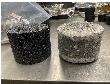
Figure 21. Cantabro Specimens Before and After Testing
