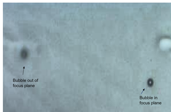
Figure 4.10: Bubble in focus plane versus bubble out of focus plane
