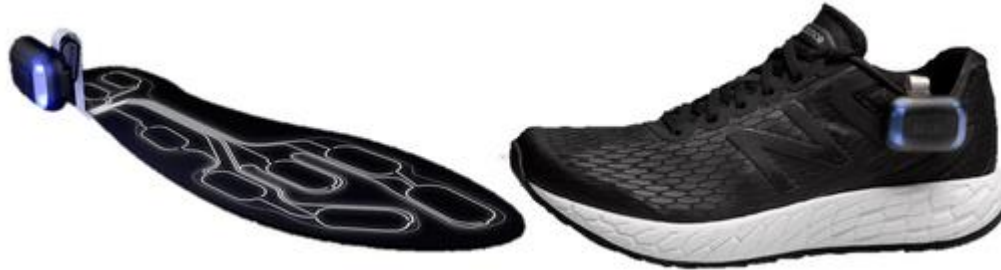
Fig. 9: An insole system offered by ARION. The insole system is pictured on the left, whereas the right visual demonstrates the inertial momentum unit that hangs outside the shoe when worn [58].
