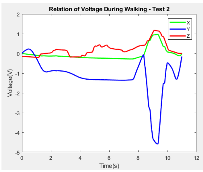
Fig. 128: The resulting voltages of the back system analysis point during practical testing during the second test of walking with the insole system.
