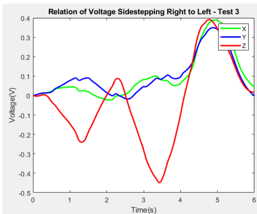
Fig. 166: The resulting voltages of the middle system analysis point during practical testing during the third test of sidestepping from right to left with the insole system.
