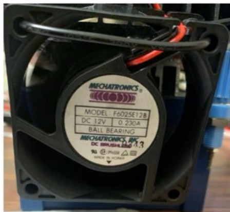
Figure 2.29: Cooling Fan Attached to the heatsink
