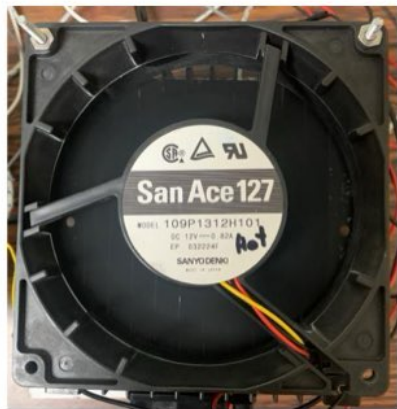
Figure 2.28: Dissipating fan attached to the Cooling channel
