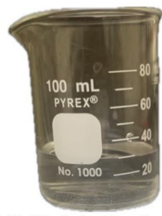
Figure 3.17: 30 ml of water collected by the prototype for 2 hours and 30 min.
