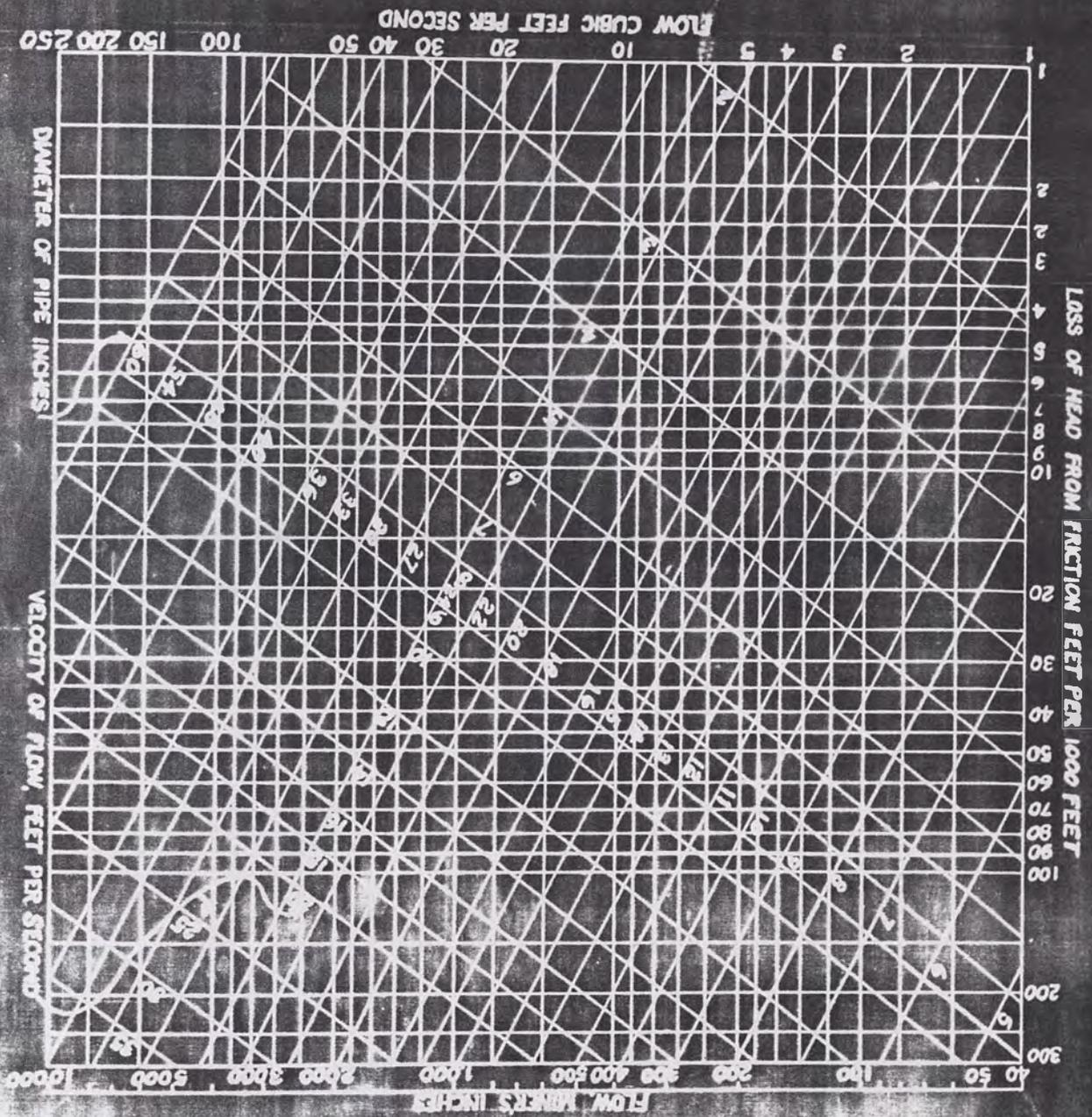
a 22-foot head loss may not be serious. In tight gravel, however, it probably would be economical to use just the 16-inch and 18-inch diameters, or possibly to construct the whole line of 18-inch pipe. If the total available head were 200 feet, the smaller pipe probably would prove satisfactory, as the percentage of loss would only be one half as much as with a 100-foot head.
