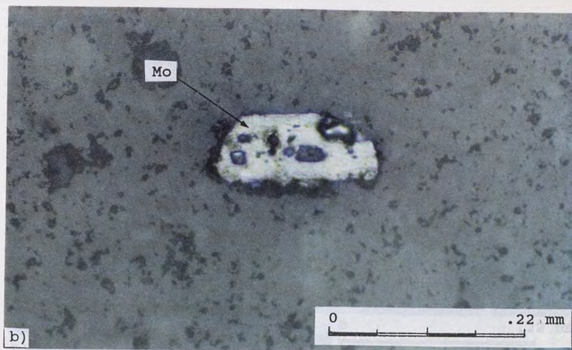
Figure 17. a) Chalcopyrite and bornite. Textural relations are unclear, but bornite appears to be replacing chalcopyrite along fractures (section Cr-286a). b) Disseminated molybdenite grain (section 7).
