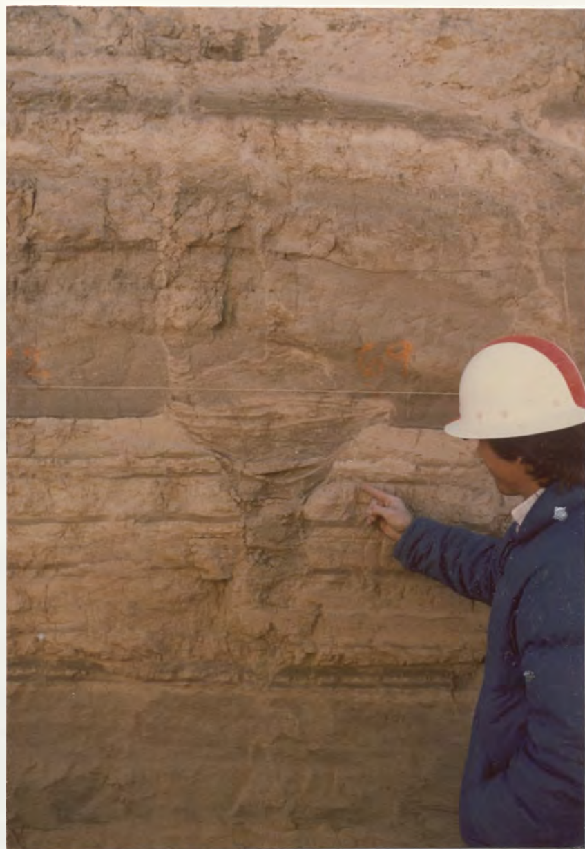
FIGURE 34. View of the stratigraphic unit that contains most of the mud volcanos exposed by the Little Lake trench.
