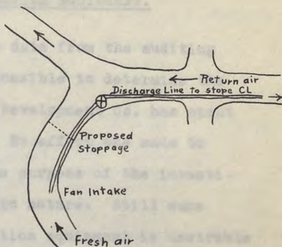
Set-up fan CK, 1000 level. Discharged air may re-enter fan intake.
