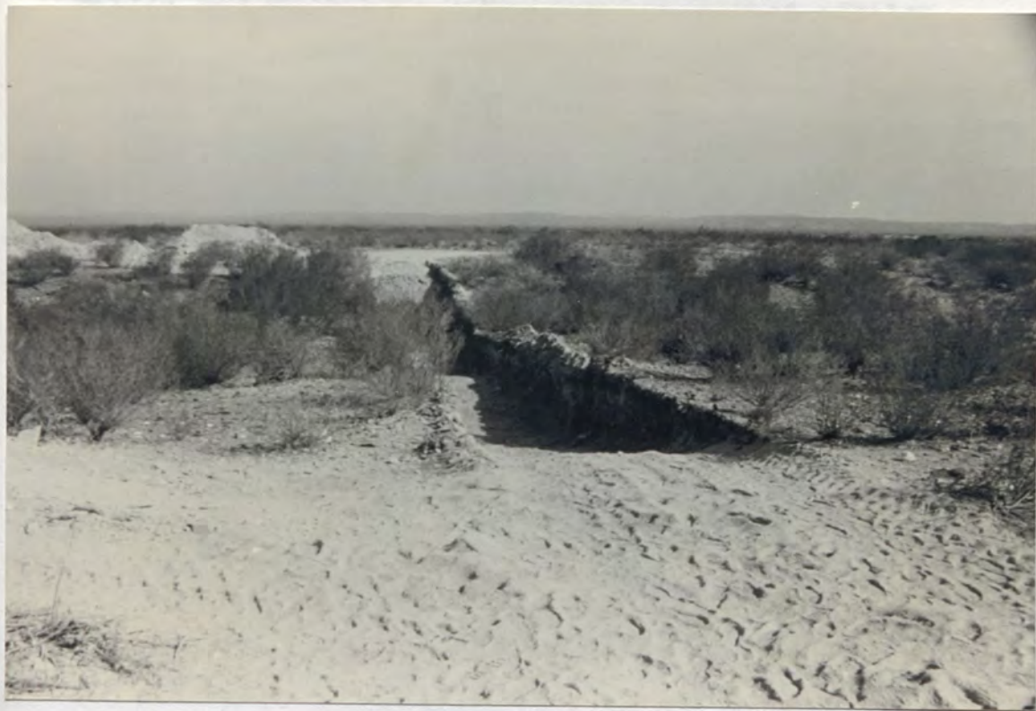
Figure 29. Photograph of Trench 10 across a graben of the Niquizanga fault zone. Location before trench emplacement is shown in Figure 28. See Trench log 10.
