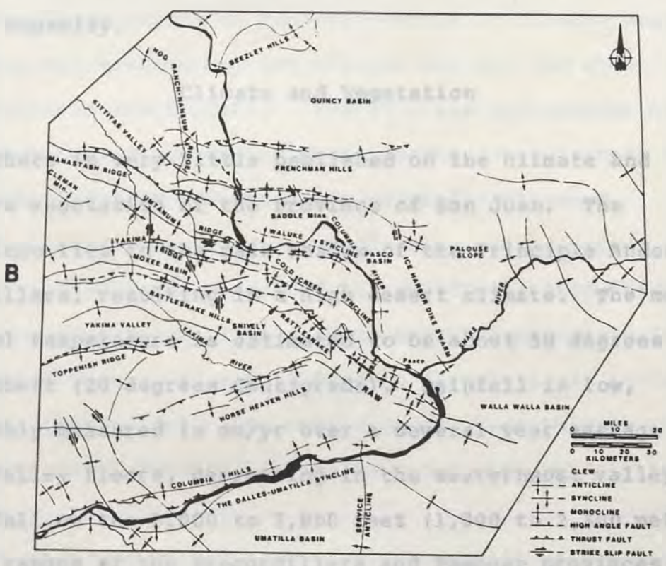
Figure 2. A. Location map of the Columbia Plateau and the aerial extent of the Columbia River Basalt Group. Also shown are the Pasco Basin and the major structural subdivisions within the Columbia Plateau (Reidel et. al., 1990). B. Structural elements of the Yakima fold/thrust belt. RAW is the Rattlesnake-Wallula alignment (Reidel et. al., 1990).
