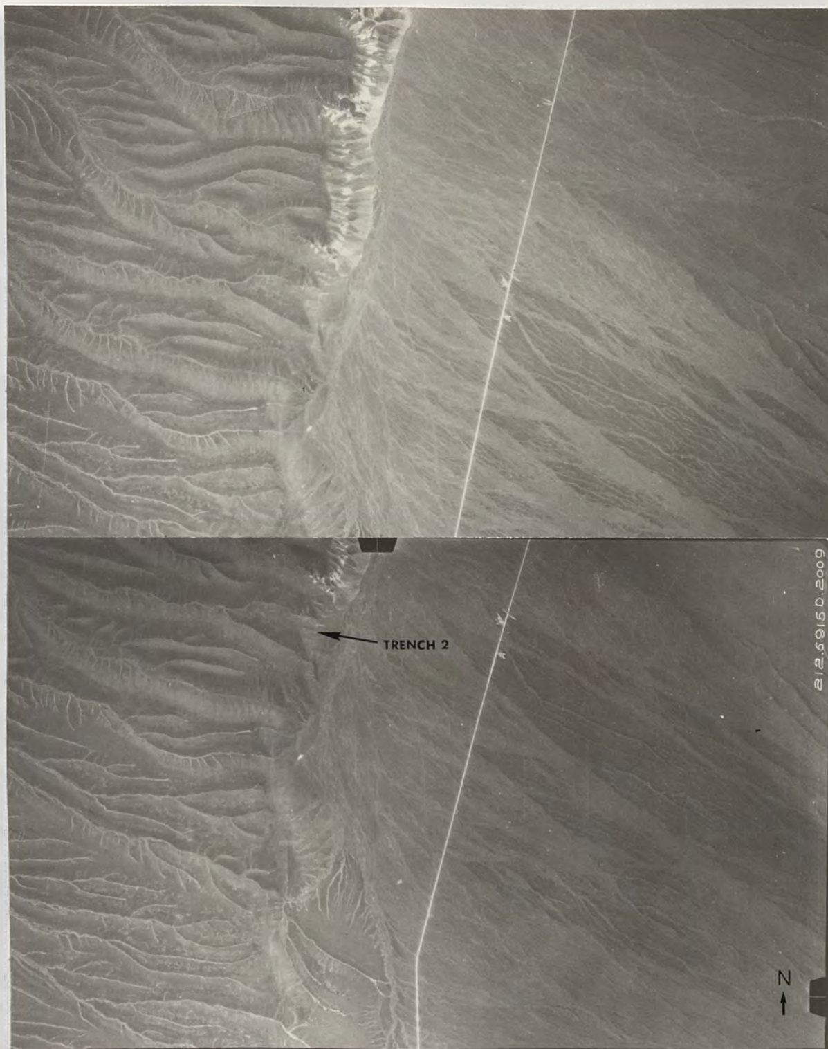
Figure 10. Stereographic aerial photographs of the El Tigre fault in the area of trench 2, about 30 miles (48 km) north of the San Juan river. Scale is approximately 1:40,000.
