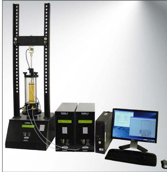
Figure 3-3. Geocomp's triaxial system
