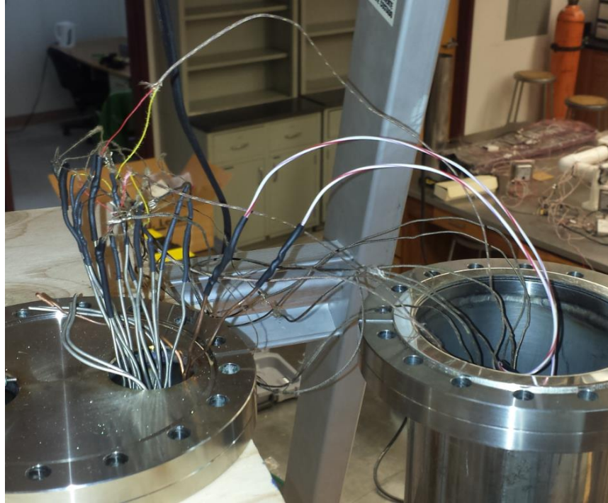
Figure 3.7. Thermocouple and power wires connected to vacuum side of feedthrough.
