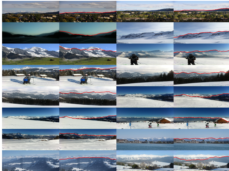
Figure 4.13: Examples of faulty detection with average error more than five pixels: sample images (column 1 & 3), solution found by fusion approach (column 2 & 4).
