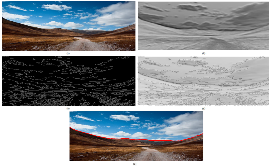
Figure 4.11: Fusion based horizon detection: (a) query image, (b) DCSI, (c) MSEE Edges, (d) fused DCSI, (e) detected horizon (red boundary).
