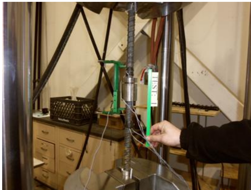
Figure 2-17 HC tensile test specimen set-up
