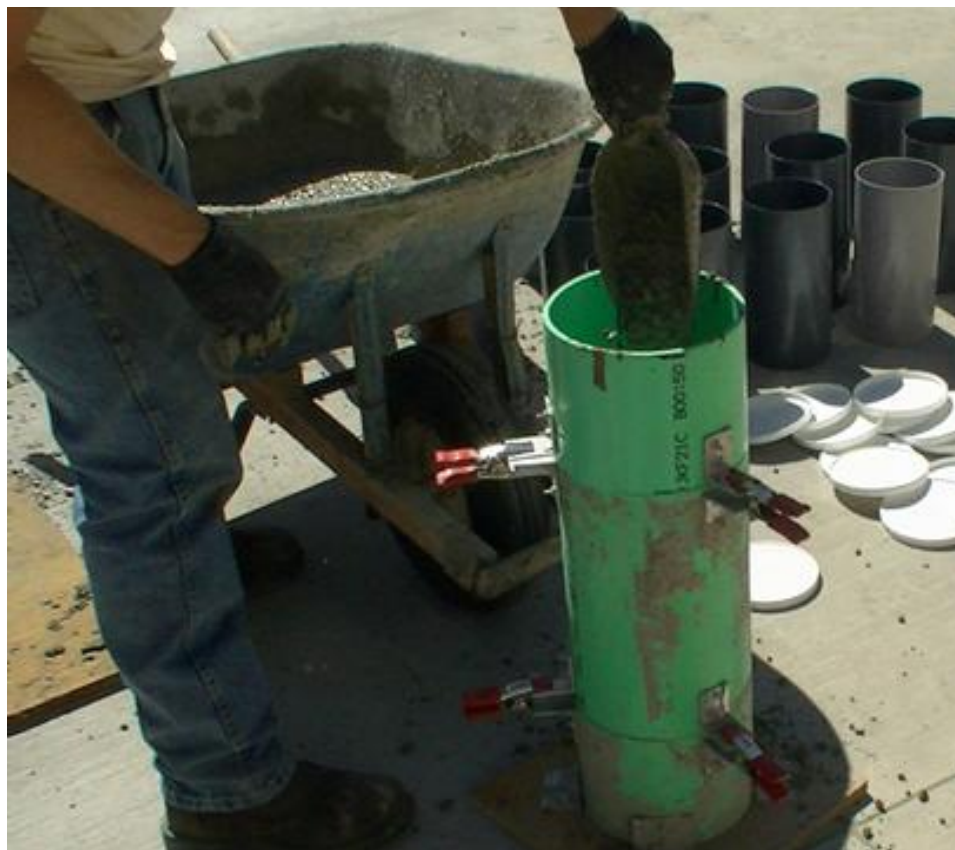
Figure 3-42 Filling SCC segregation column
