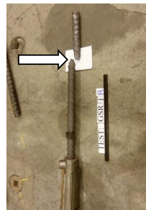
(b) Location of rupture
