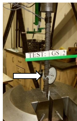
(b) Location of rupture
