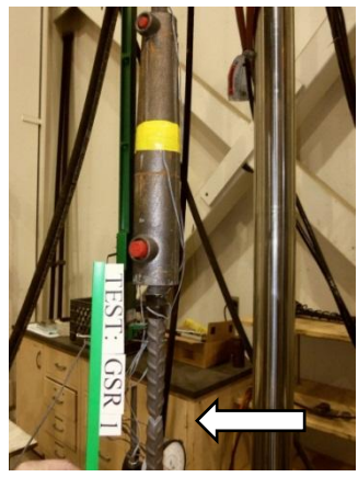
(b) Location of rupture
