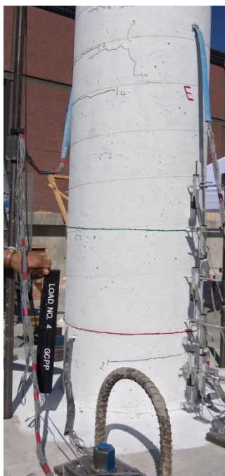
(a) South-east face second pull cycle of 0.25% drift
