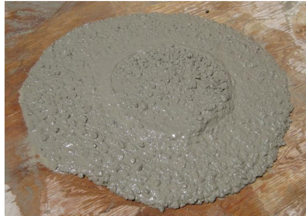
(b) Slump flow test 2: d_{\text{avg}} = 20.3\text{in} [516mm] and VSI = 0.0
