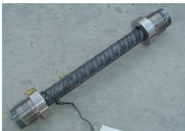
Figure 3-29 Transition bar with male threaded ends
