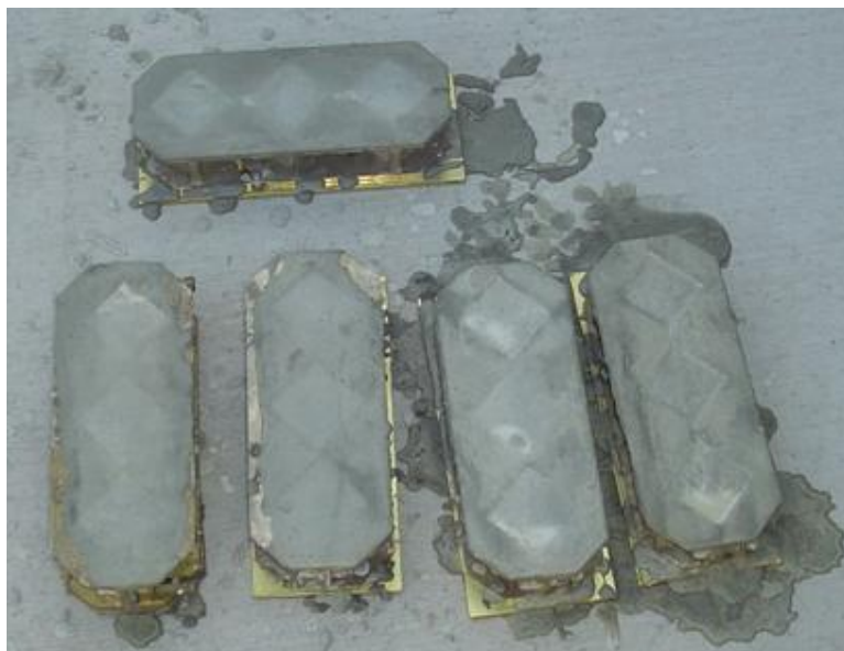
Figure 3-38 Casting of grout cubes
