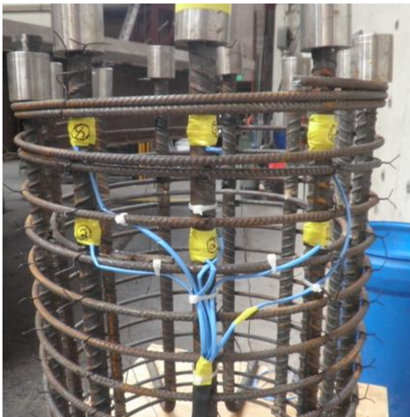
Figure 3-55 HCNP instrumented footing dowel cage
