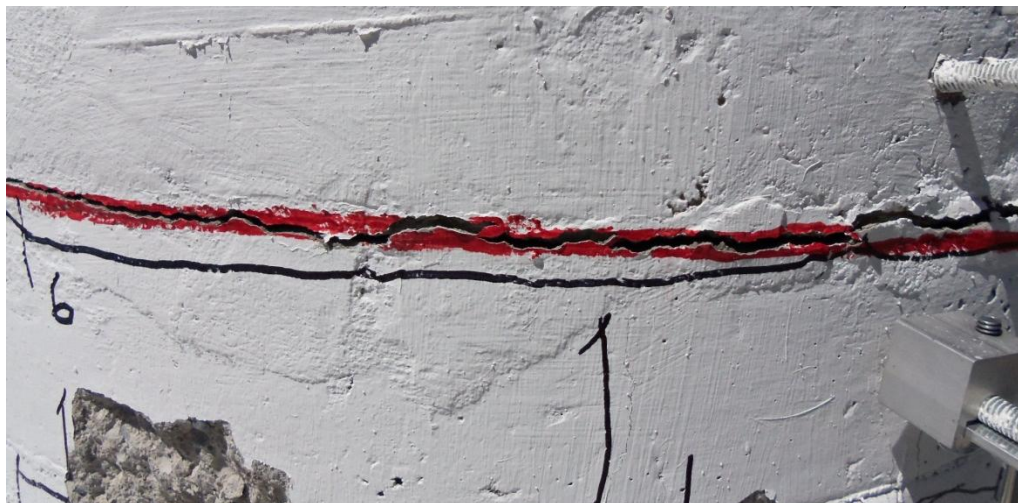
(a) Concentrated crack ( \approx 0.14 in [3.5 mm]) at pedestal-column joint during first pull cycle
