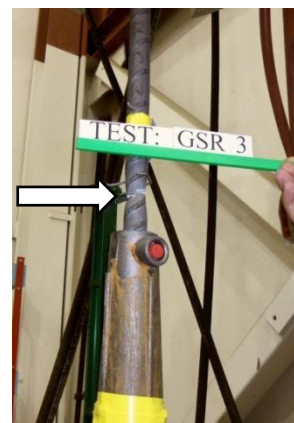
(b) Location of rupture
