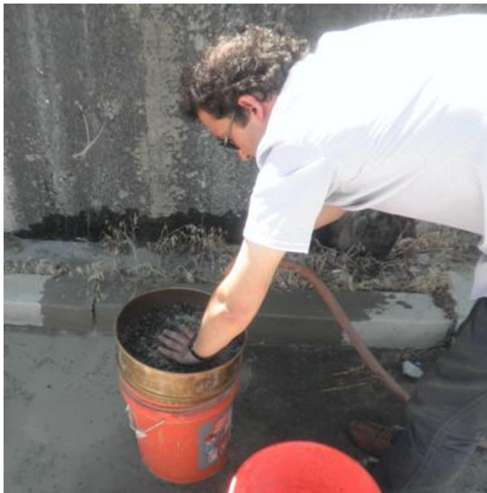
Figure 3-44 Sieving segregation column contents
