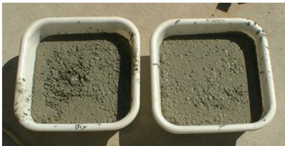
Figure 3-43 Collection of segregation column top and bottom contents
