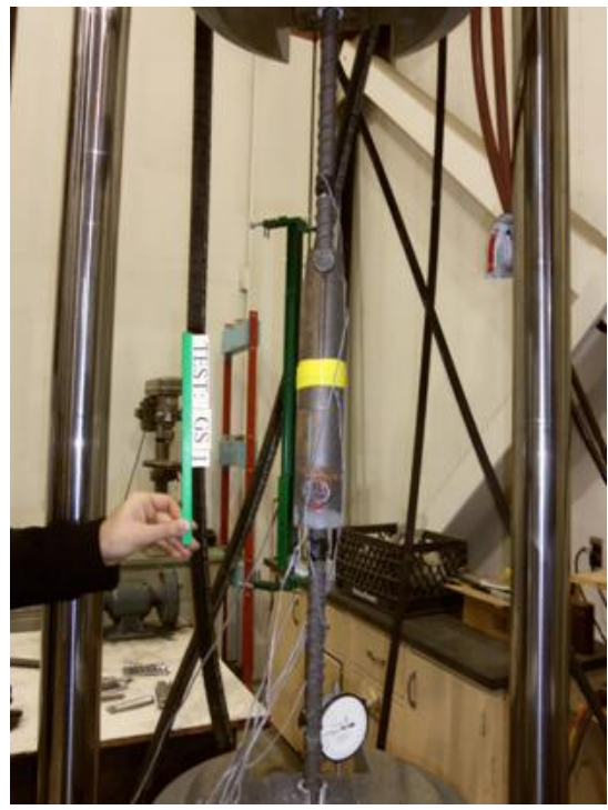
Figure 2-19 GC tensile test specimen set-up
