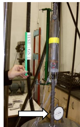
(b) Location of rupture
