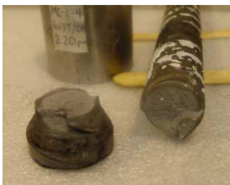
Figure 2-9 Failure of upset headed splices other than bar rupture
