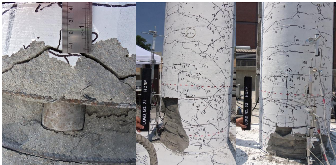
(a) West face first push cycle (b) South-west face second push cycle (c) East face second pull cycle
