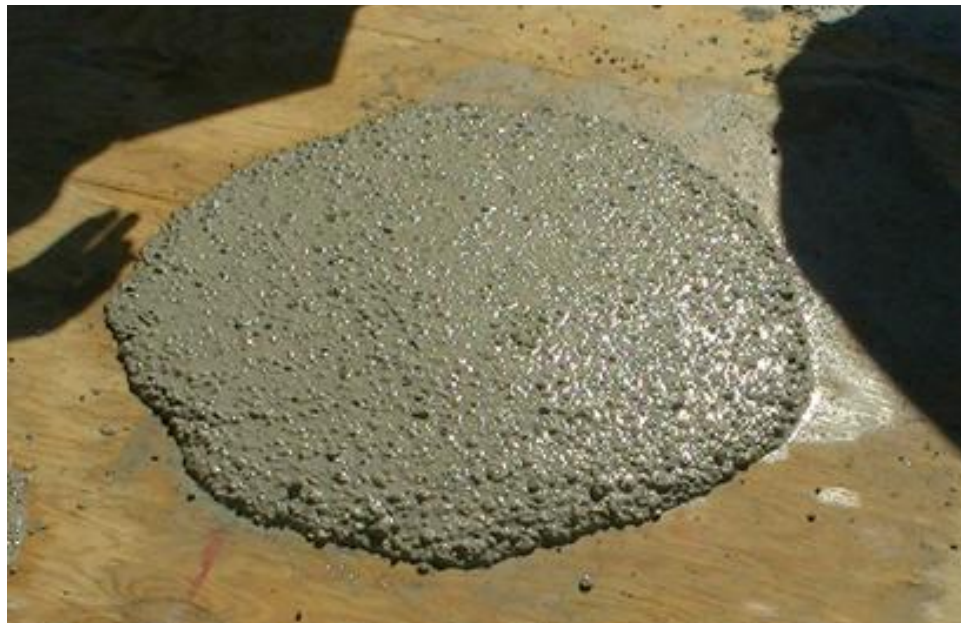
Figure 3-41 Final slump-flow test of SCC
