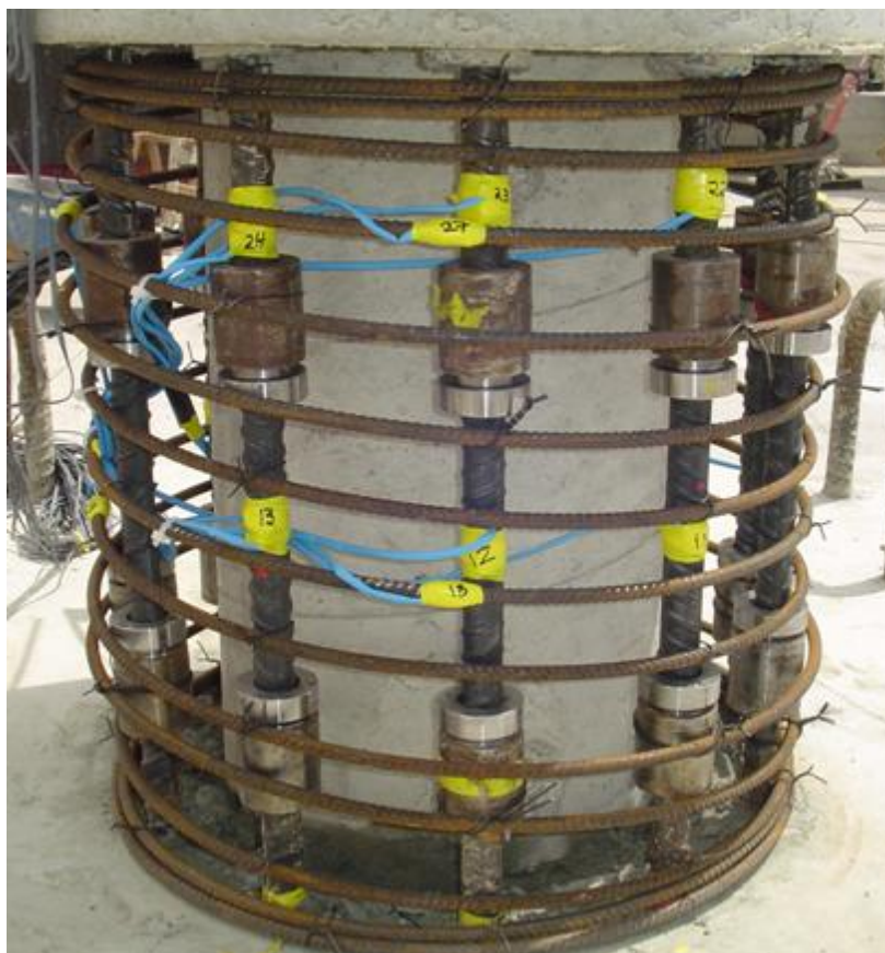
Figure 3-57 Instrumentation of closure region
