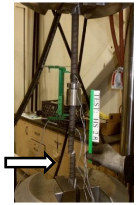
(b) Location of rupture
