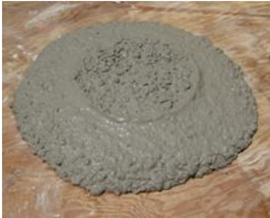
(a) Slump flow test 1: d_{\text{avg}} = 17.3\text{in} [439mm] and VSI = 1.0
