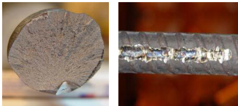
(a) Fracture at the first screw
