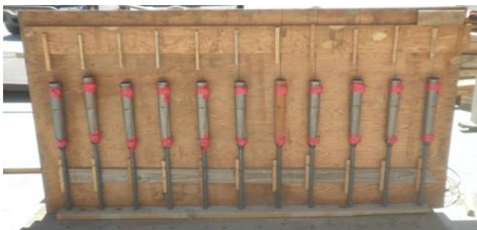
Figure 2-14 Grouted coupler test specimens ready for grouting
