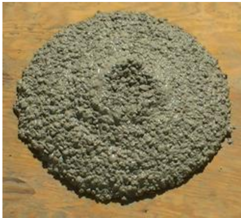
(a) Slump flow test 1: d_{\text{avg}} = 16.5\text{in} [419mm] and VSI = 1.0
