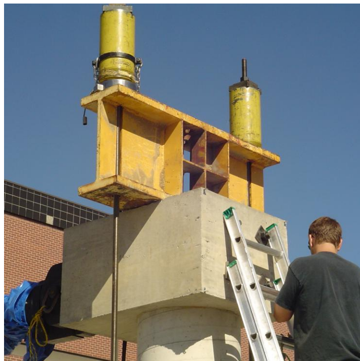
Figure 3-101 Spreader beam and loading rams
