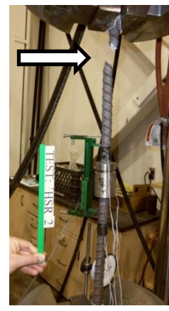
(b) Location of rupture
