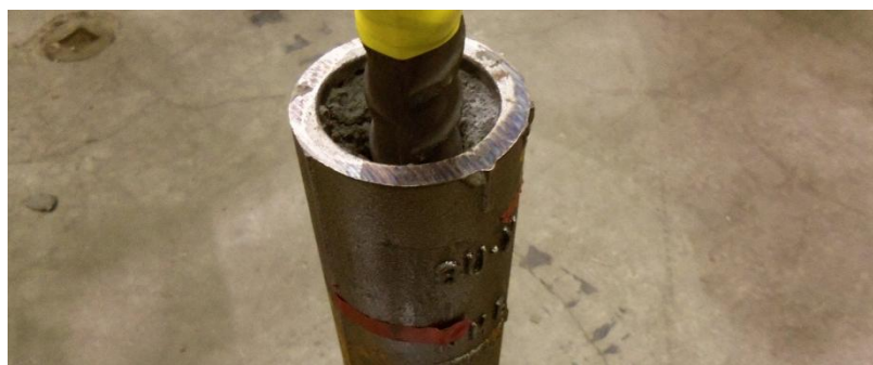
Figure 4-85 Grout cone due to strain penetration
