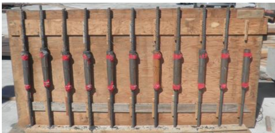
Figure 2-15 Grouted coupler test specimens after grouting and bar insertion
