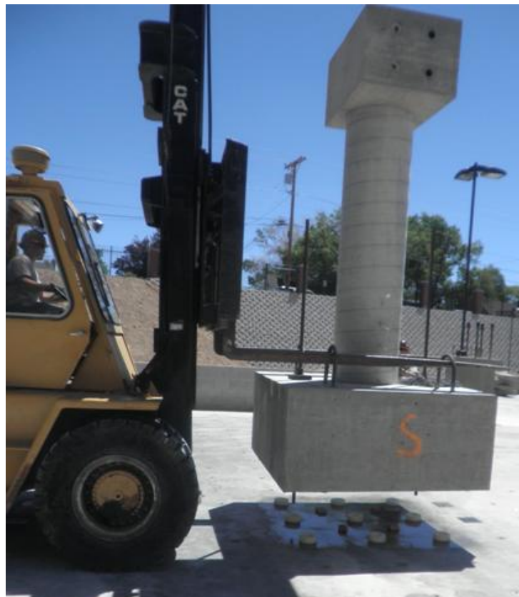
Figure 3-99 Placement of column model
