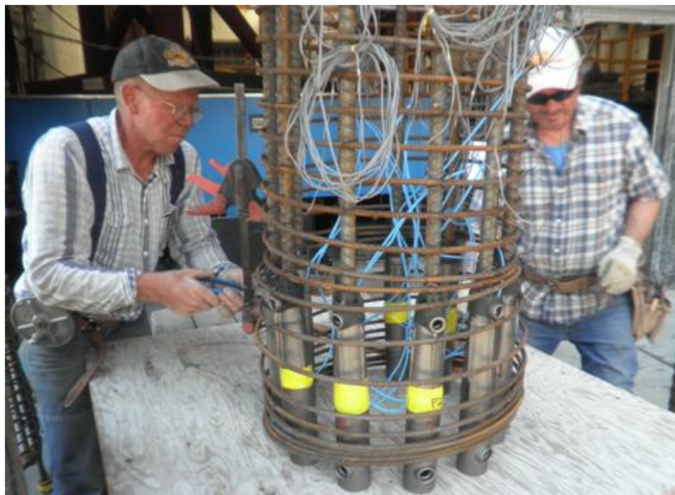
Figure 3-72 Tying spiral around GCNP coupler region
