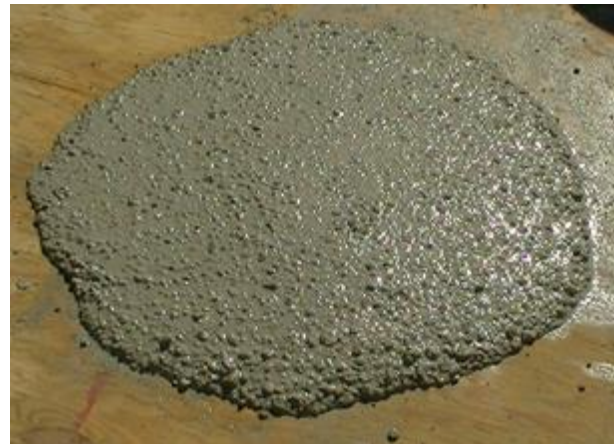
(b) Slump flow test 3: d_{\text{avg}} = 25.3\text{in} [643mm] and VSI = 0.0
