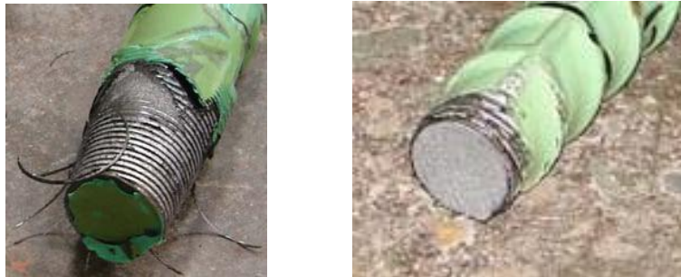
(a) Stripping of the threads (b) Fracture at the threads Figure 2-10 Failure of tapered thread splices other than bar rupture
