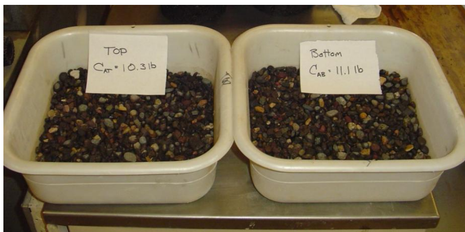
Figure 3-45 Segregation column contents after sieving
