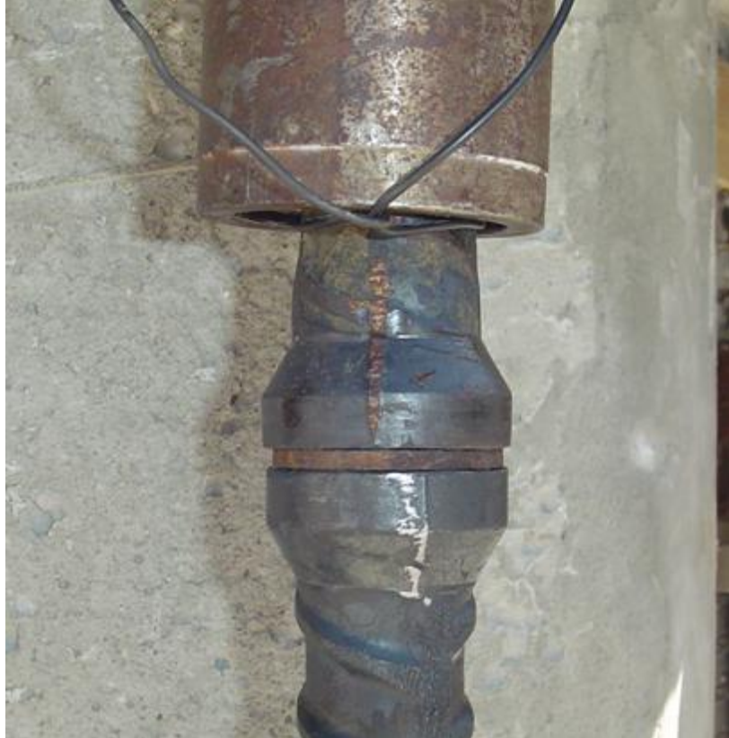
Figure 3-32 Spacer inserted between upper heads
