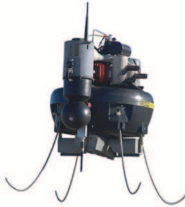
Figure 1.2: Honeywell T-Hawk MAV [2].
