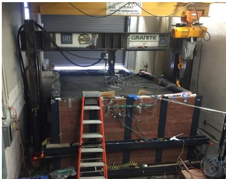
Figure 6.34. Photo. The full-scale pavement/soil testing facility at the University of Nevada Reno.
