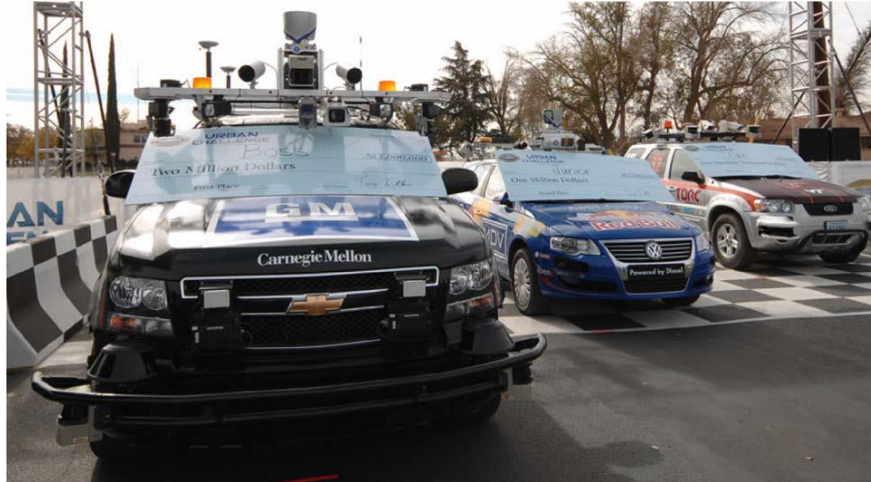
Figure 9 Testing Vehicles in DARPA Urban Challenge 2007, with Sensors on Top
