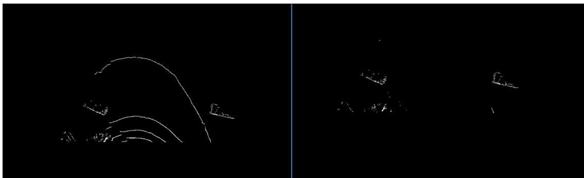
Figure 17 Data Frame After Outlier Removal (left) and Data Frame After Ground Plane Removal (right)
