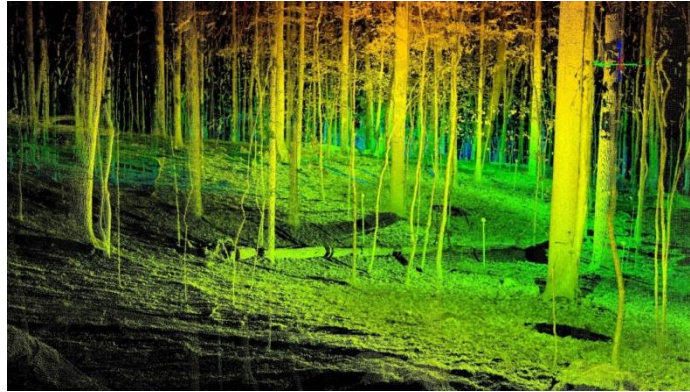
Figure 1 Terrestrial LiDAR Image
