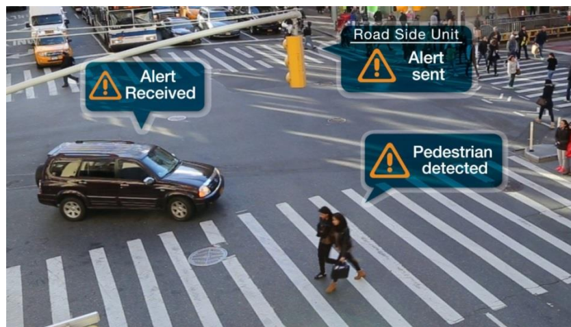
Figure 42 Connected Vehicle Application Example
