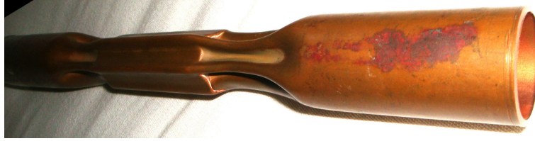
Figure 3.13: A Cu pipe with a 3 mm wall was placed inside the bore of the solenoid before pulsing to 16 T within a rise time of 400 \mu s. There is a solid Al bolt inside the pipe. The induced Eddy currents generated a \mathbf{J} \times \mathbf{B} pinching effect that squeezed the pipe around the bolt. If the field can bend metal, there is a concern that it can move optical mounts place near the solenoid.
