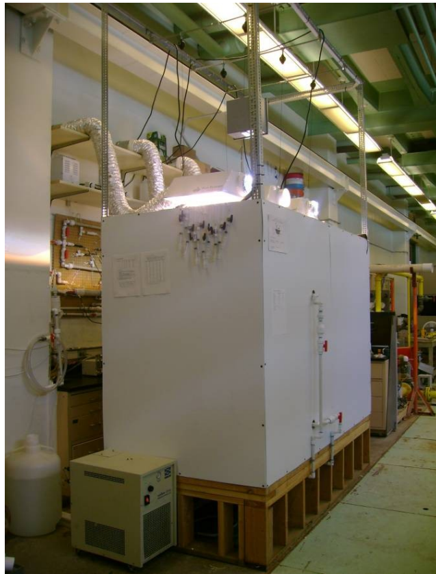
Figure 5: Salinity gradient solar pond with three high-intensity discharge lamps, each consisting of a halide/sodium bulb in order to replicate natural sunlight. Each bulb is powered by a ballast.
