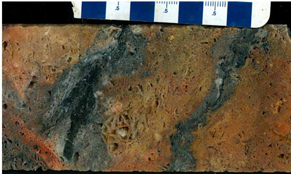
Figure 24. Hand sample of oxidized and leached gossan with sparse relict pods of pyrite encapsulated in quartz (scale in cm).
