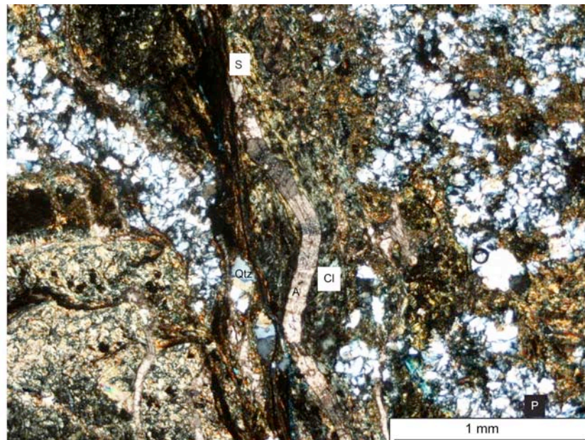
Figure 19. Skarn sample from ~900' below the RBM pit made up of pods of phlogopite (P) + chlorite (Cl), and pods of quartz (Qtz) + serpentine (S) veined by late ankerite (A) (Sample RBD0601-910.5, PPL, mineralogy verified with EDS).
