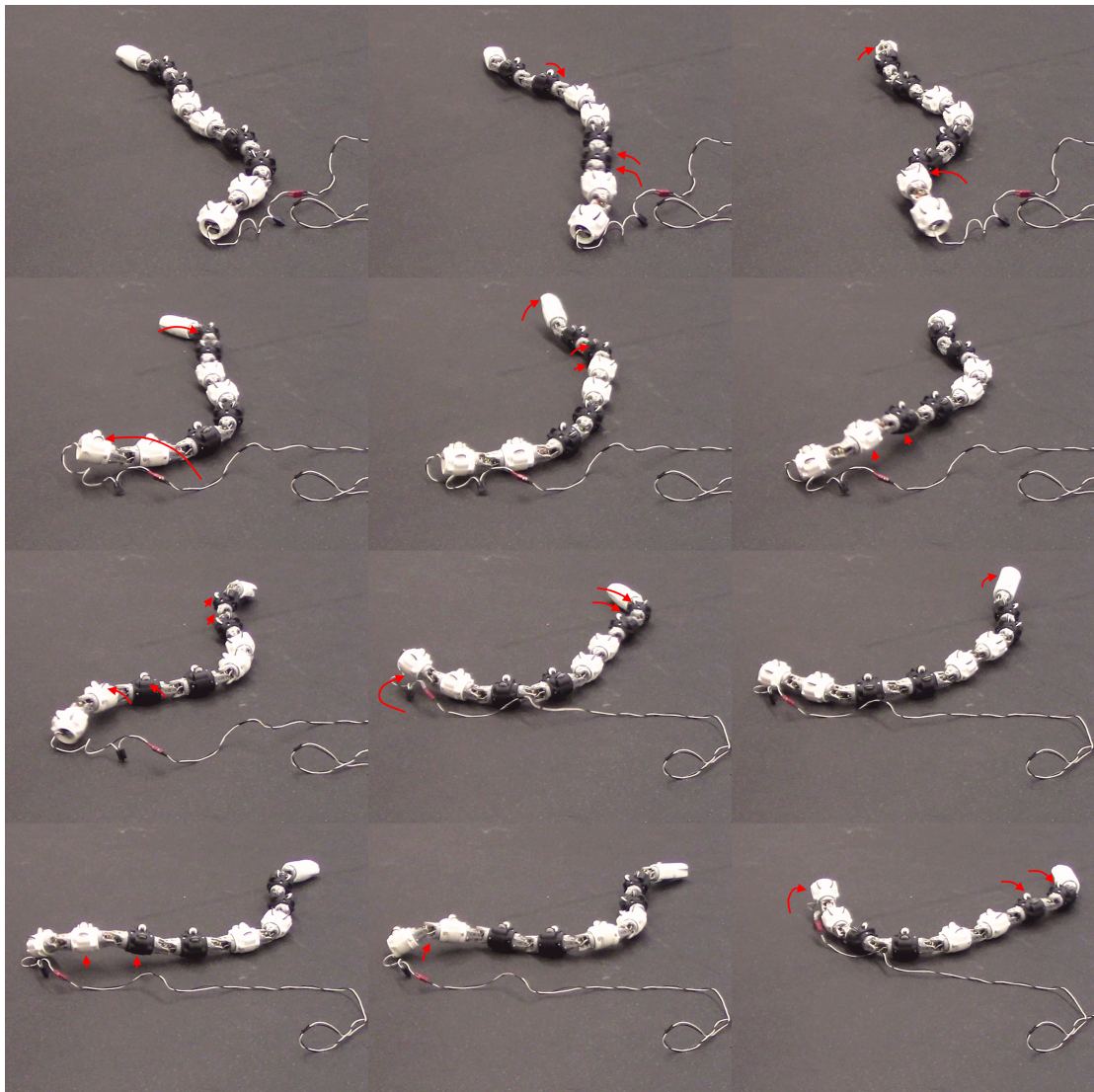
Figure 3.1.8: Differential sidewinding. Images were taken in increments of 0.5 sec, from left to right, then top to bottom.
