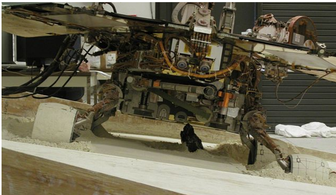
Figure 1.2.1: Laboratory attempt to replicate conditions of the accidentally immobilized Spirit Rover. Courtesy NASA/JPL-Caltech [36].
