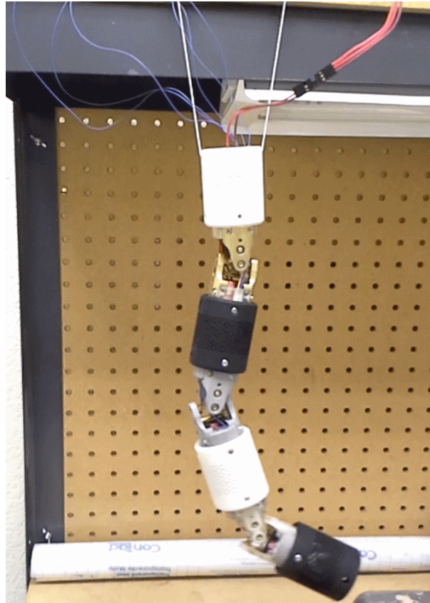
Figure 4.1.1: Three segments consisting of original (Prototype I) robot snake parts suspended on string for testing.
