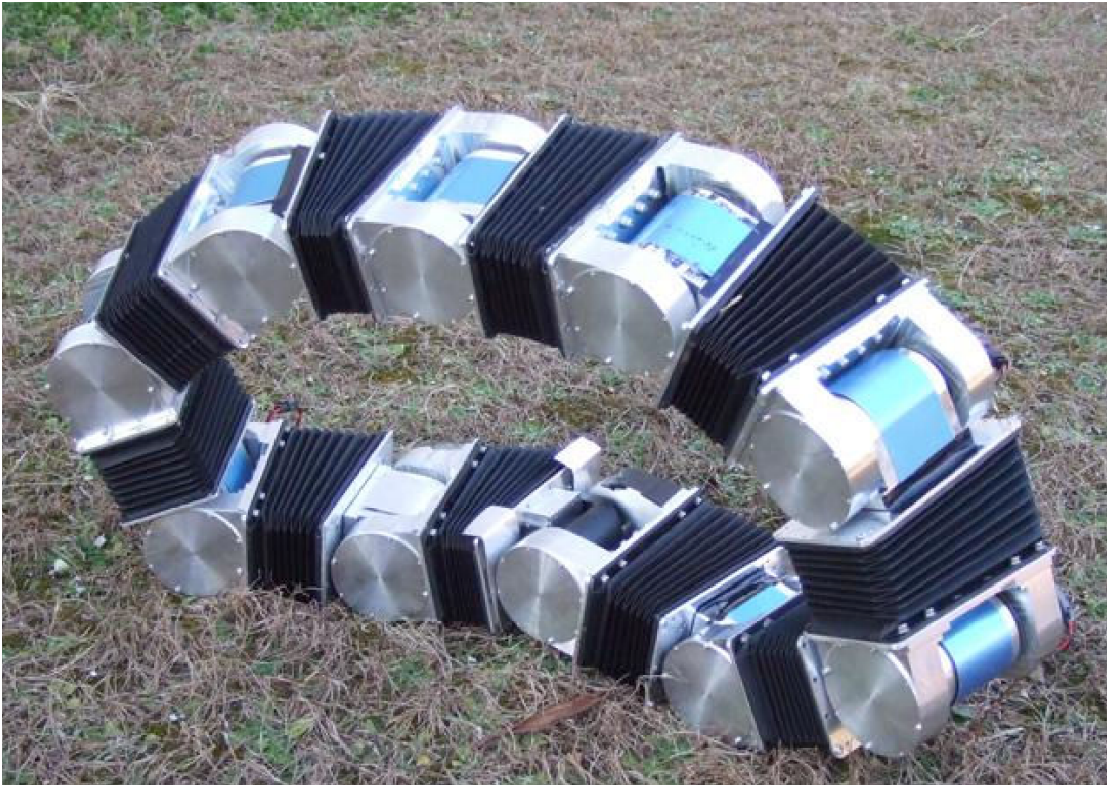
Figure 2.2.5: ACM-R7, with its body formed into a loop. Courtesy of Tokyo Institute of Technology.
