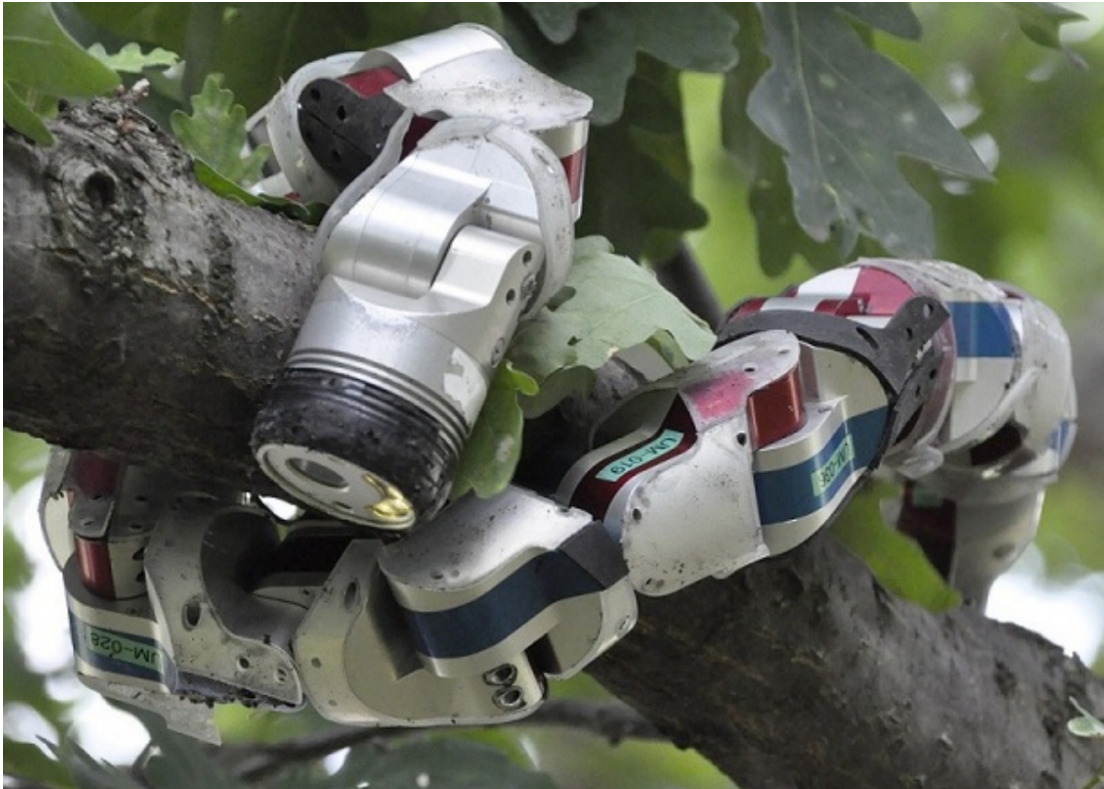
Figure 2.2.8: Unified Snake Robot. Courtesy of Carnegie Mellon University.
