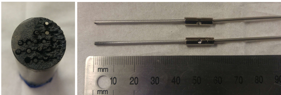
Figure A2.4: 1/16" dia x 2" long Mg_2Ni rods machined via EDM from bulk Mg_2Ni (left) and MgNi_2 rods connected to Ni rods via Ni plated crimp connectors prior to use in the reference electrodes used in this study.
