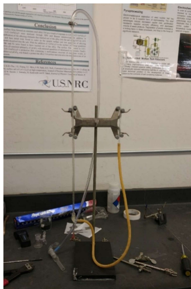
Figure A6.1: Gas measurement apparatus used for determination of H 2 volume generated from reaction of Li with H 2 O. The salt sample is placed in a sealed reaction vessel with 10 mL of DI H 2 O that is connected via a flexible tube to the top of a 5 mL burette, which is filled with water. The pressure inside the closed system is maintained at atmospheric pressure via a movable reservoir connected to the bottom of the burette via a second piece of flexible tubing.
