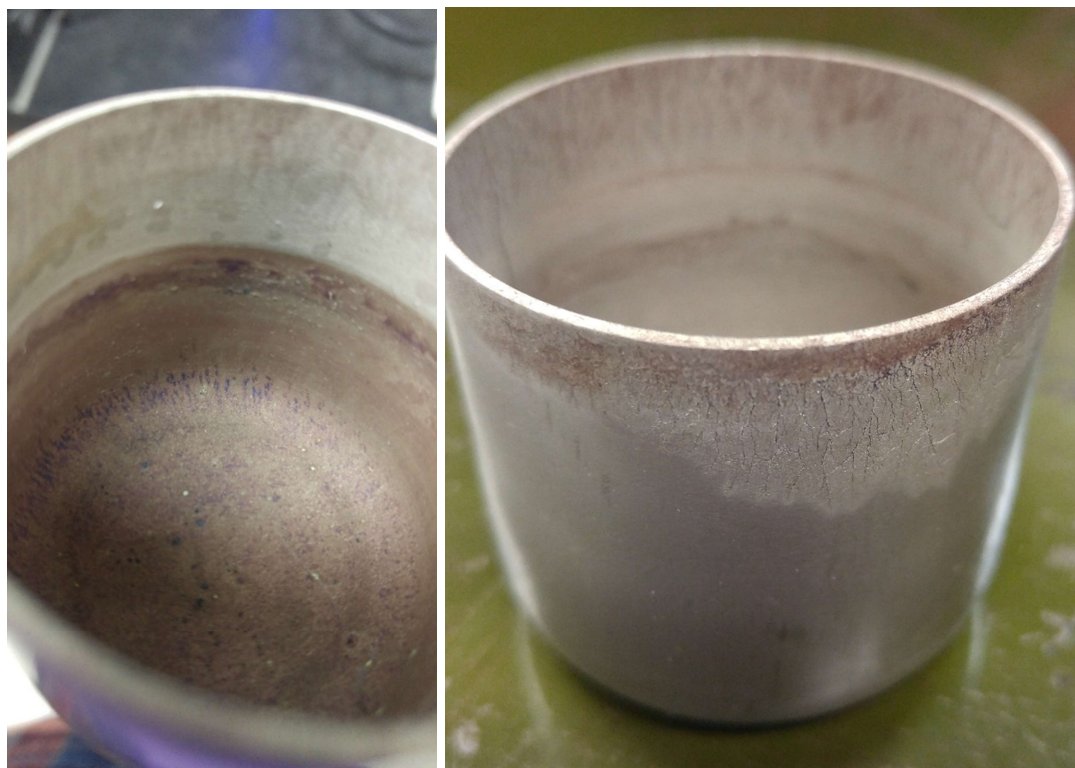
Figure A5.1: Image of Ni Crucible used to expose I625 samples to \text{LiCl-2wt\%Li}_2\text{O-1wt\%Li} for 1000hr. Severe degradation was observed, both above and below the melt line. Below the melt line, precipitation of corrosion products was observed which show a purple color. This may be indicative of lithium molybdenum purple bronze ( \text{Li}_{0.9}\text{Mo}_6\text{O}_{17} ), but further analysis would need to be conducted to determine the composition of this corrosion product. Above the melt line, dendritic structures were observed to be etched into the crucible wall, with apparent growth up and over the side of the crucible. This can be most readily observed in the figure on the right.
