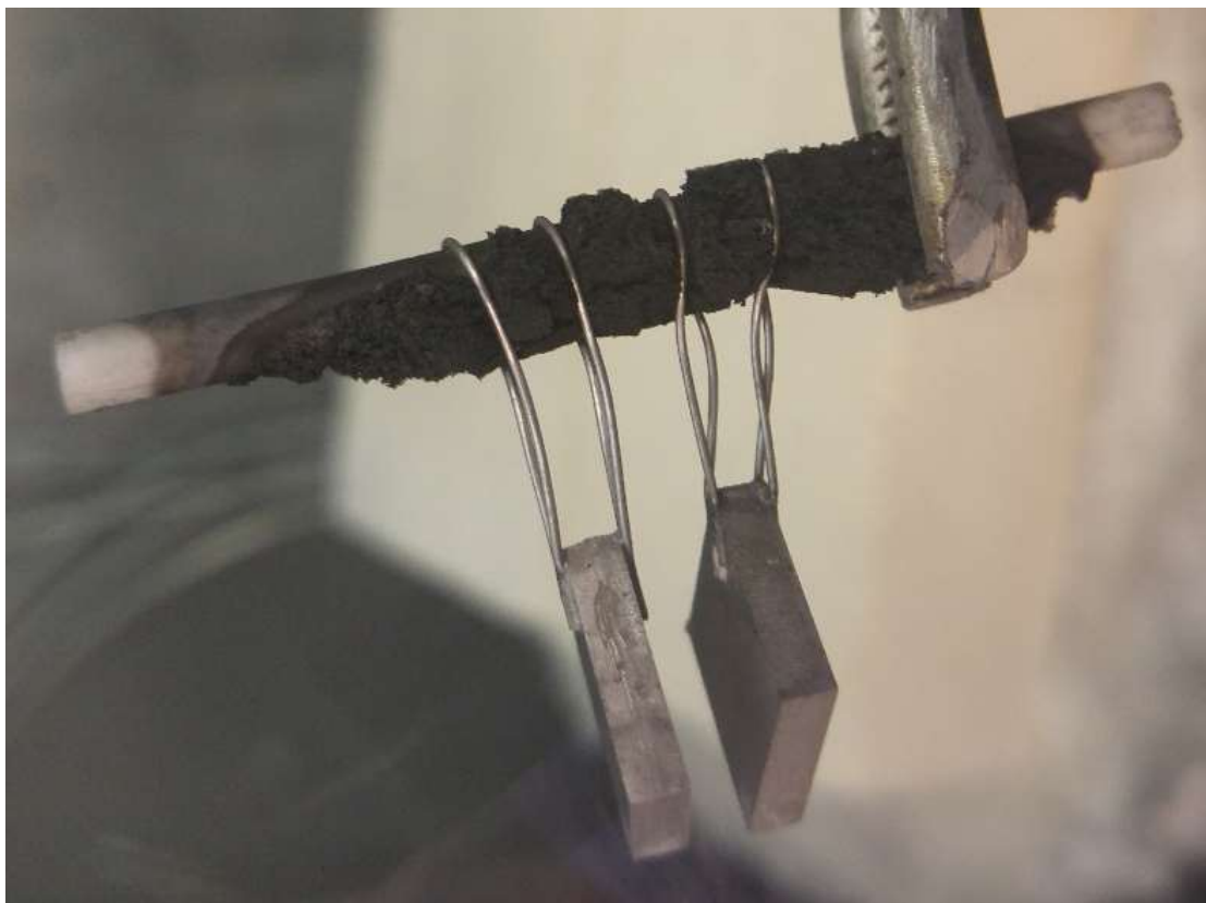
Figure A3.3: Degradation of alumina ( \text{Al}_2\text{O}_3 ) rod used to hang samples for exposure testing in \text{LiCl}-2\text{wt}\%\text{Li}_2\text{O}-0.6\text{wt}\%\text{Li} for Chapters 2, 3, and 4, demonstrating the incompatibility of \text{Al}_2\text{O}_3 with the conditions in this system. The attack shown here was from the vapor phase above the salt, and was caused by metallic Li and Na vapors (Na is present as the major impurity in all Li compounds used for this study). This degradation occurred in less than 72 hours, and resulted in the complete failure of 6 out of 8 identical rods, resulting in failure of these experiments.
