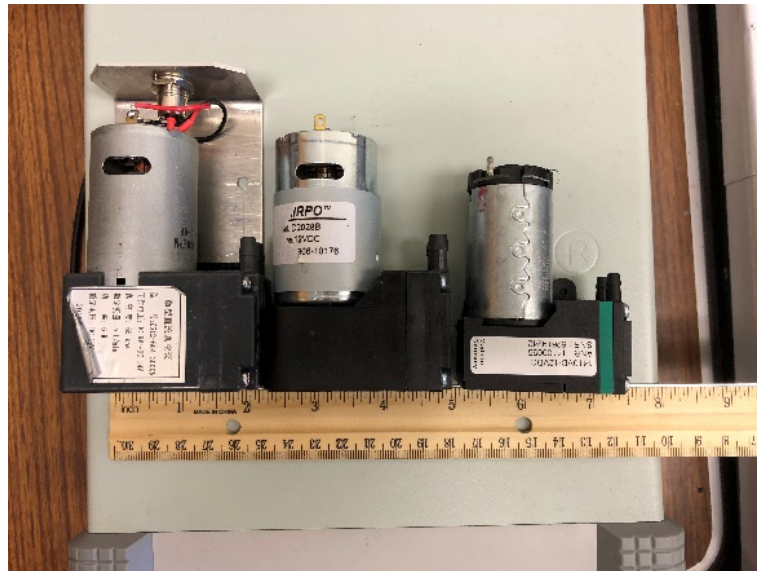
Figure 17: Small Vacuum Pumps used in Trials
