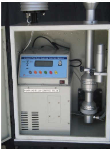
Figure 3: PEM-ADS 2.5µ/10µ Inner View (Ambient Fine Dust Sampler, 2018)
