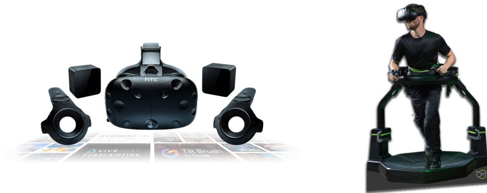
Figure 23: HTC Vive HMD (middle), controllers (bottom left and right) and lighthouse sensors (top left and right). (HTC Corporation, 2019), Omnidirectional treadmill "Omni" (Virtuix, 2019)
