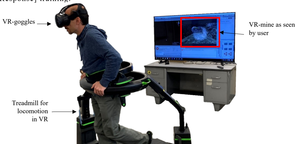
Figure 17: VR set-up for the mine evacuation simulation at LMR 155, UNR
