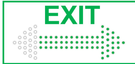
Figure 11: Schematic design of a smart exit sign with LED's that can give directional cues
