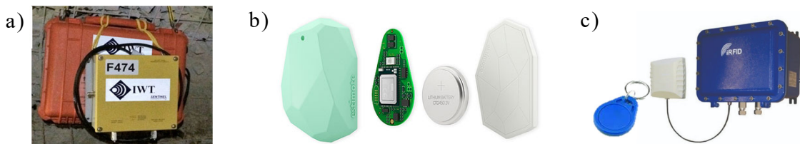
Figure 12: a) SENTINEL™ wireless station for underground by IWT®; b) components of a Beacon by Estimote Inc. and c) a RFID reader and tag (IWT, 2019; Robu, 2019; Warren, 2019; Zoon, 2019)
