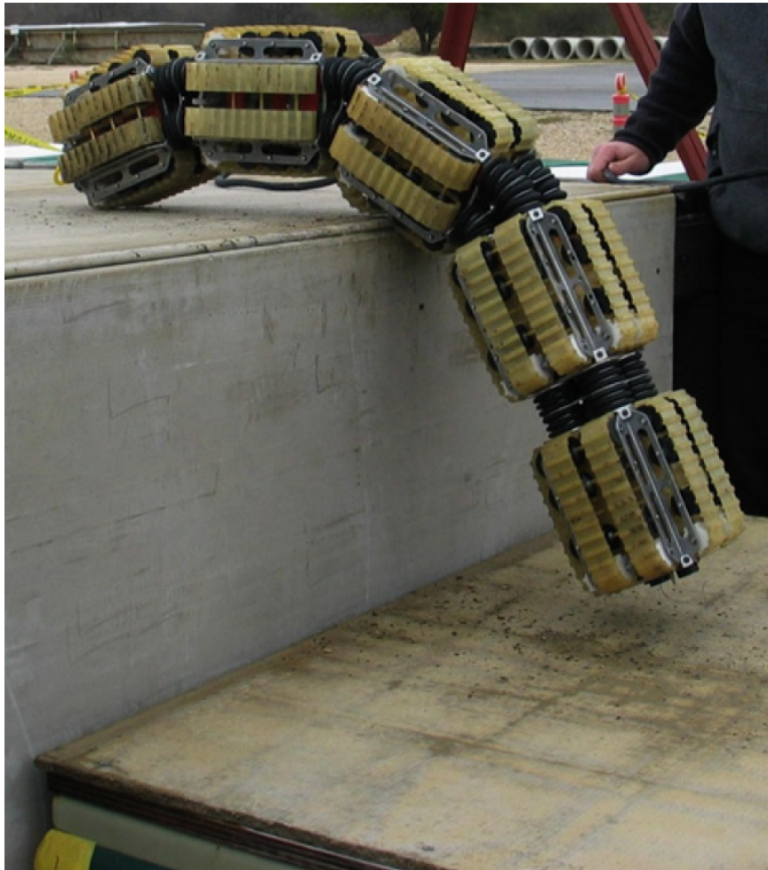
Figure 1.7: The OmniTread snake robot developed at the University of Michigan, the robot has pneumatic joints and is covered by motorized tracks [5]
