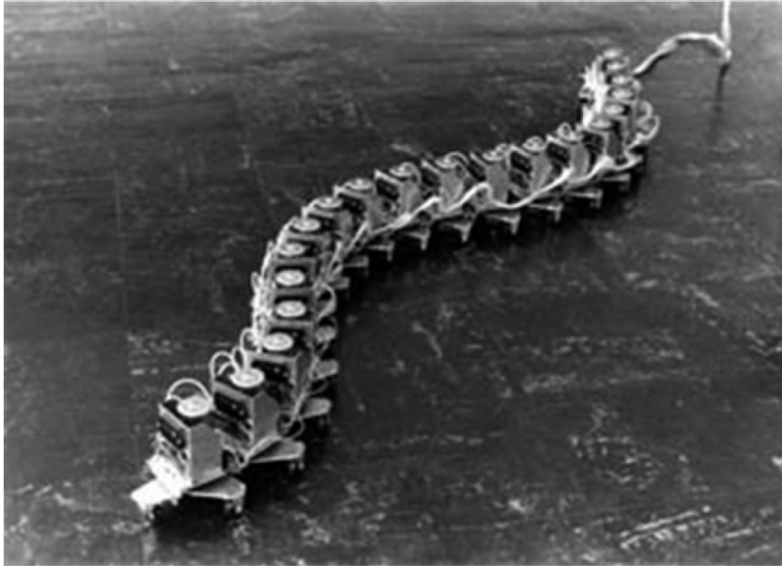
Figure 1.1: The world's first snake robot developed by Prof. Shigeo Hirose in 1972 [19]
