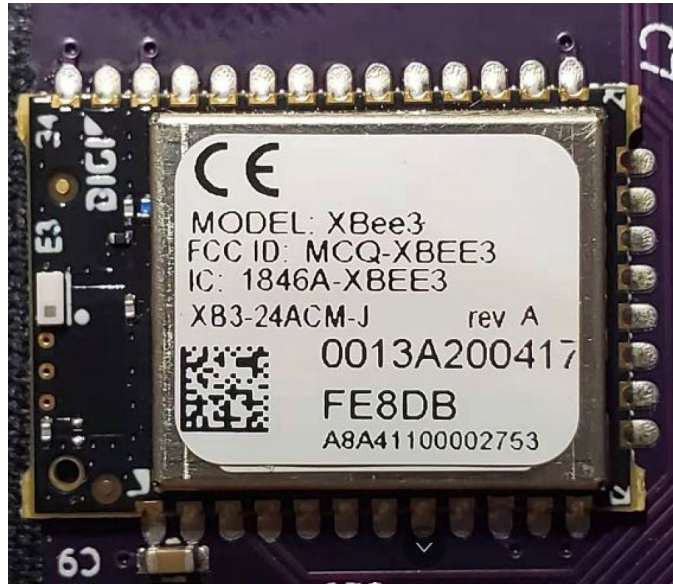
Figure 2.17: Digi XBee module allows for wireless transmission XBee module supports OTA function benefiting for snake robot reconfiguration.
