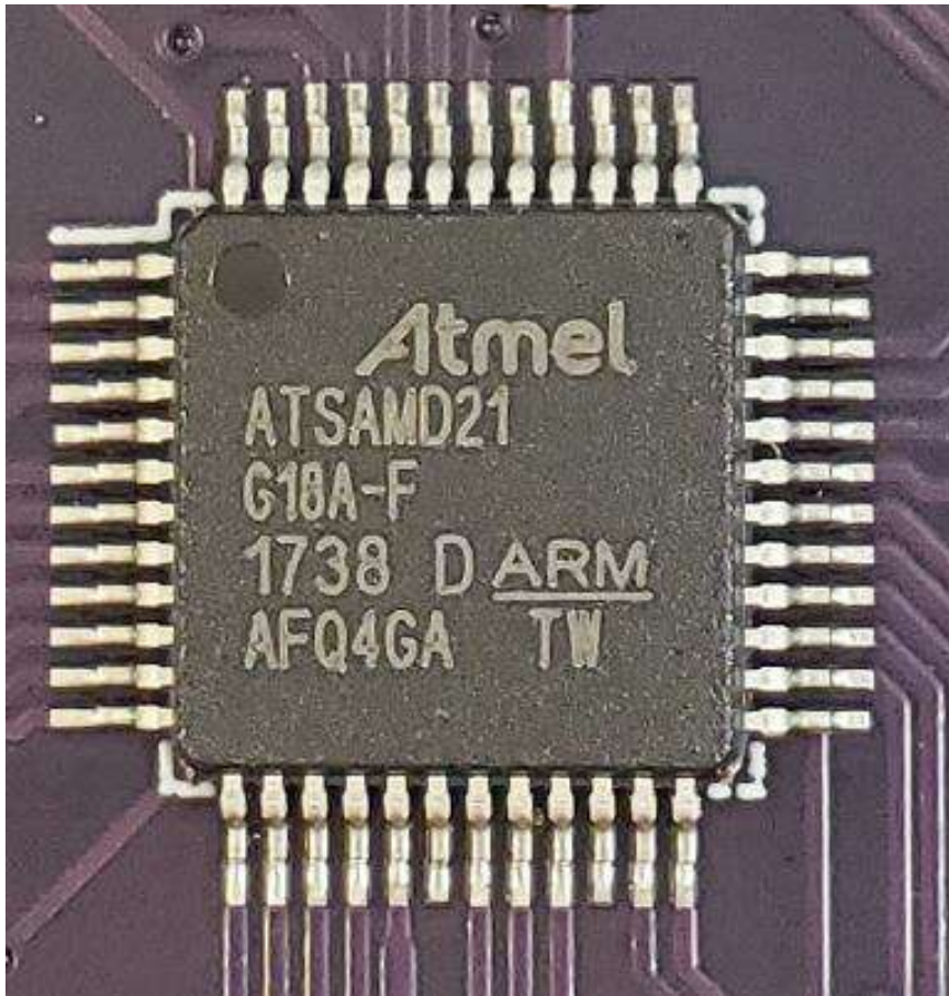
Figure 2.14: Atmel SAMD21 MCU Atmel SAMD21 provides many features to control a snake robot.
