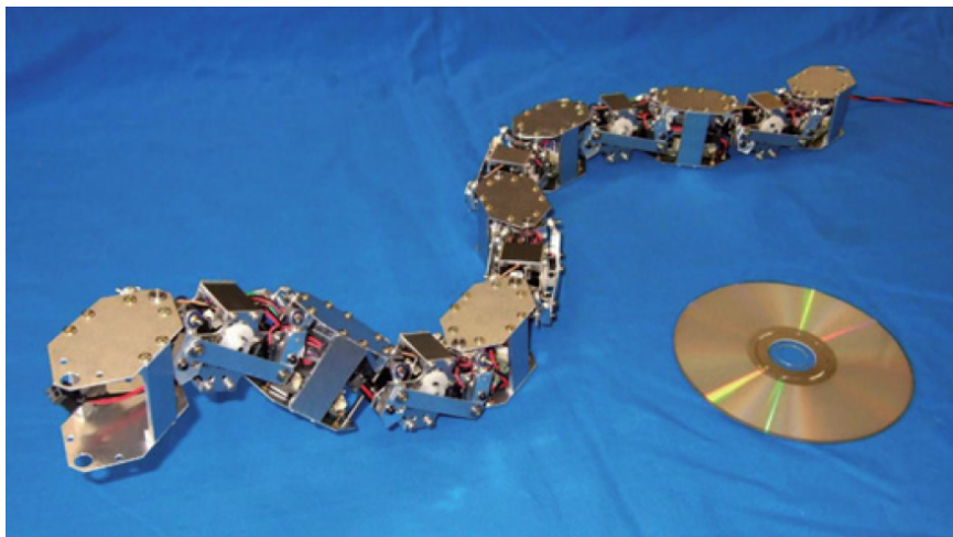
Figure 1.6: A snake robot with a miniature joint mechanism developed at Tokyo Institute of Technology [23]
