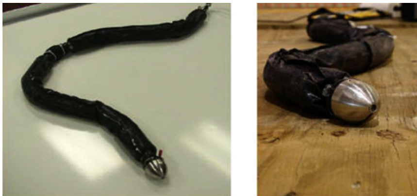
Figure 1.8: A snake robot with a skin drive propulsion system developed at Carnegie Mellon University [42]
