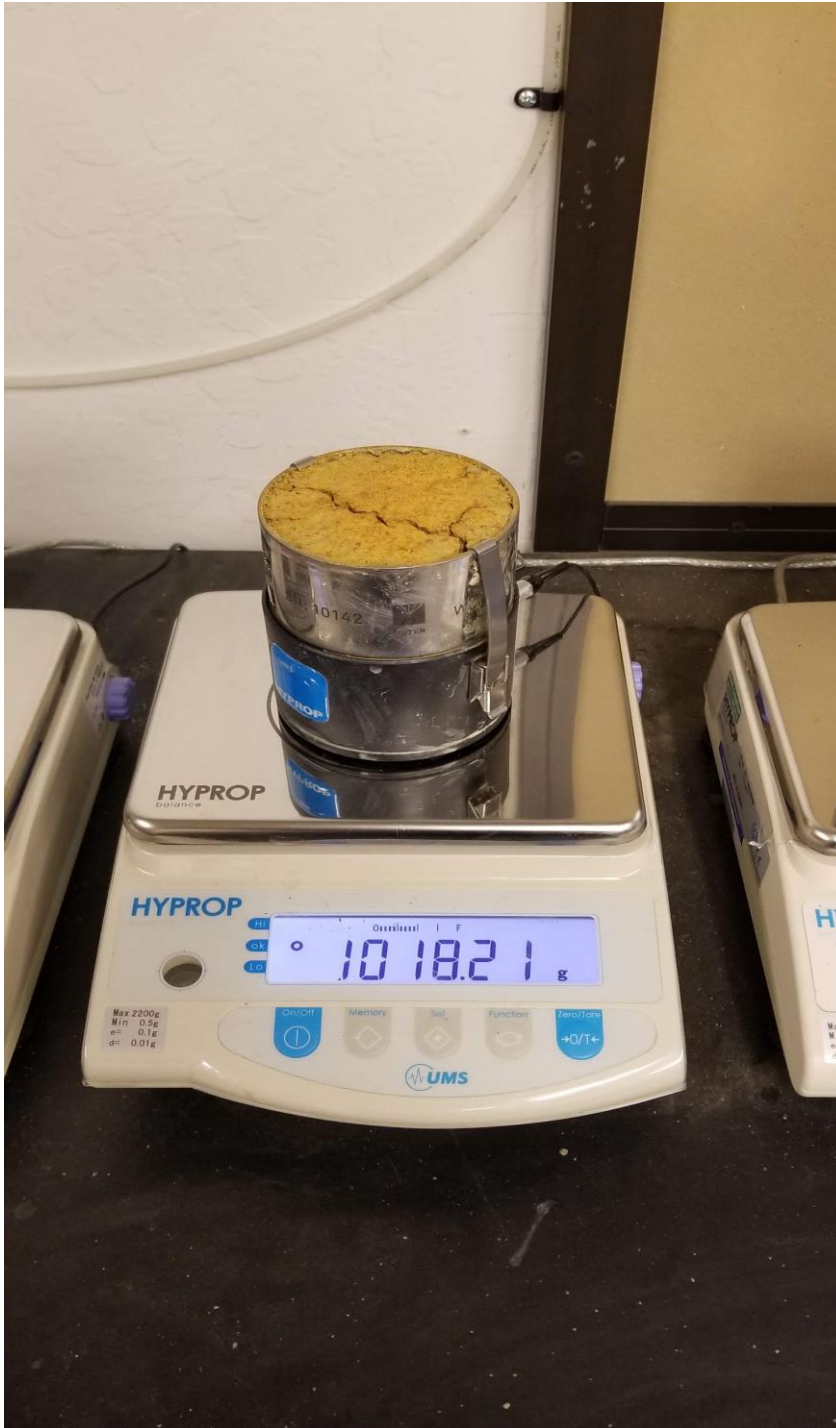
Figure 42: Picture of the HYPROP test for the first SWCC. The large crack is the soil desiccation that cause problems with the test.
