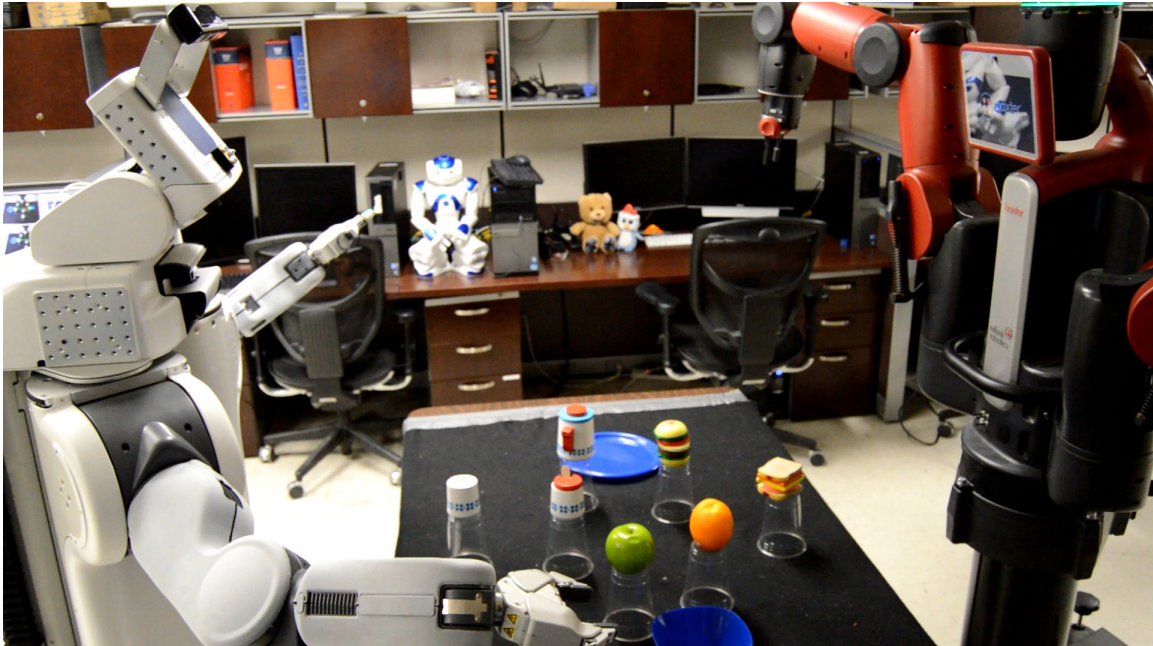
FIGURE 7.2: The setup for the multi-robot task. The PR2 (left) and the Baxter (right) are collaborating to complete a food serving task. The fruit must be placed in the bowl, the tea-set should be placed next to the bowl, and the sandwich and burger should be placed on the plate.
