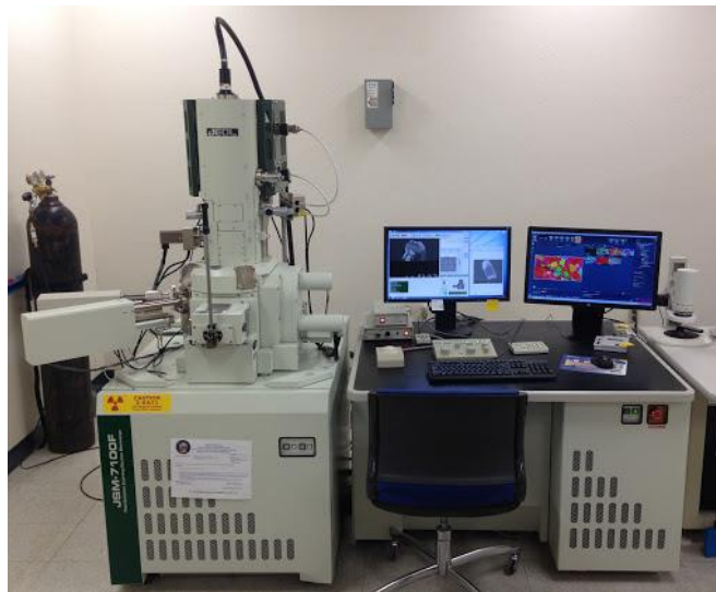
Figure 3.7: JSM-7100 FESEM Scanning electron microscope at UNR.
