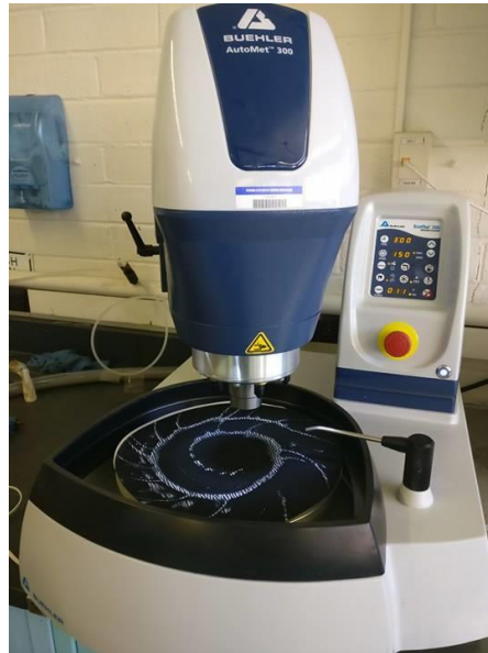
Figure 3.6: Buehler AutoMet 300 polishing machine at the Surface Engineering and Tribology lab, UNR.
