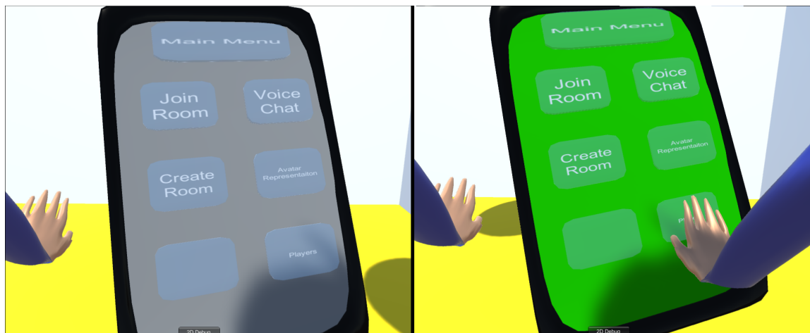
Figure 4.7: 3-D menu. When the the menu and its sub menu are enabled, the grow and translate away from the menu. Uses GameObjects for options and when a button collides with the gray area, it temporarily turns green
