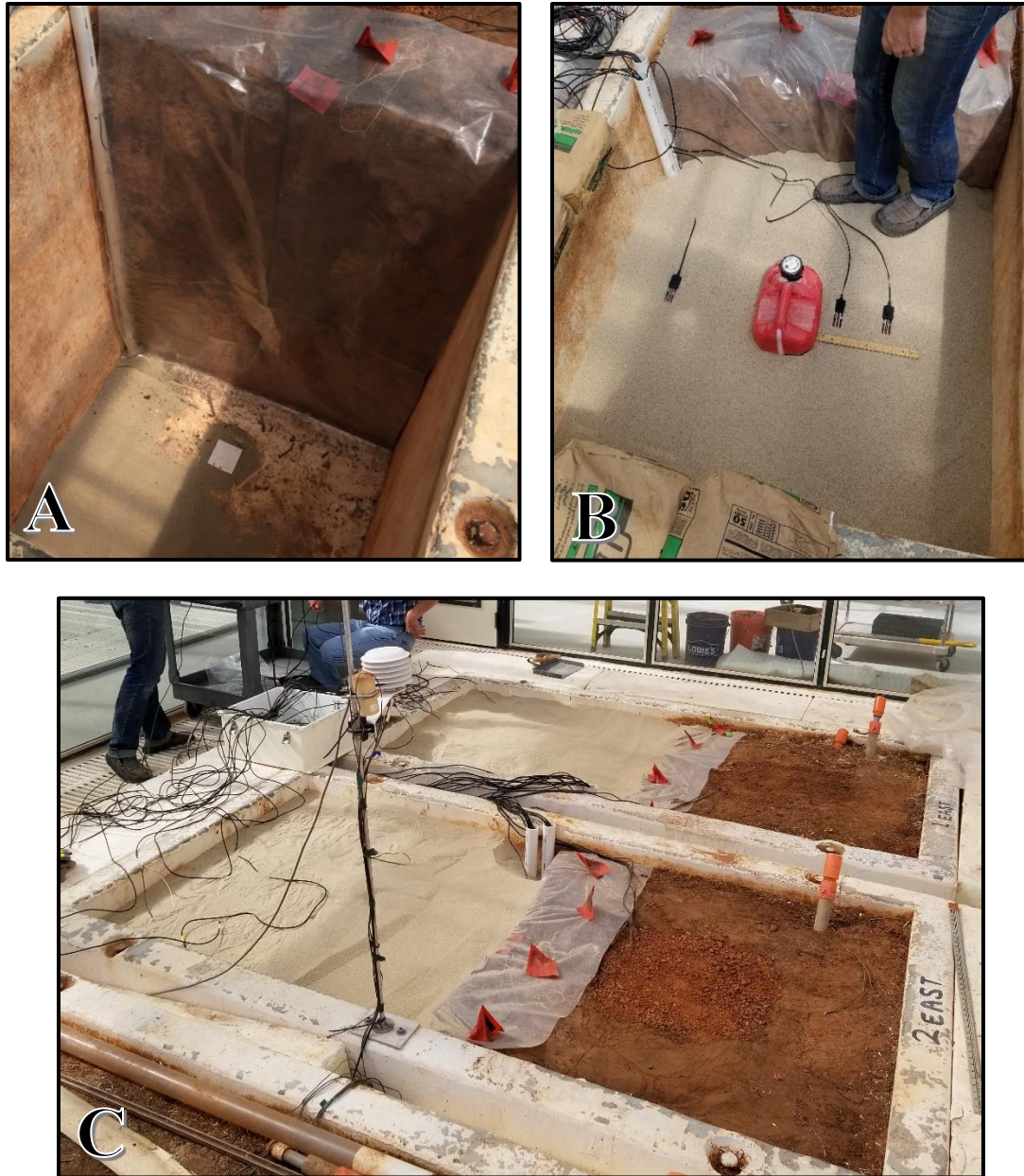
Figure 4: Panel A shows the EcoCELL plot with half of the OK soil excavated. Note the small tile placed over the drain to prevent loss of sand. Panel B shows placement of Target A and three sensors during the filling process. Panel C shows the completed experimental setup, with sensor cables routed through PVC piping to a data logger. Note the insulating foam which surrounds the soil plots.
