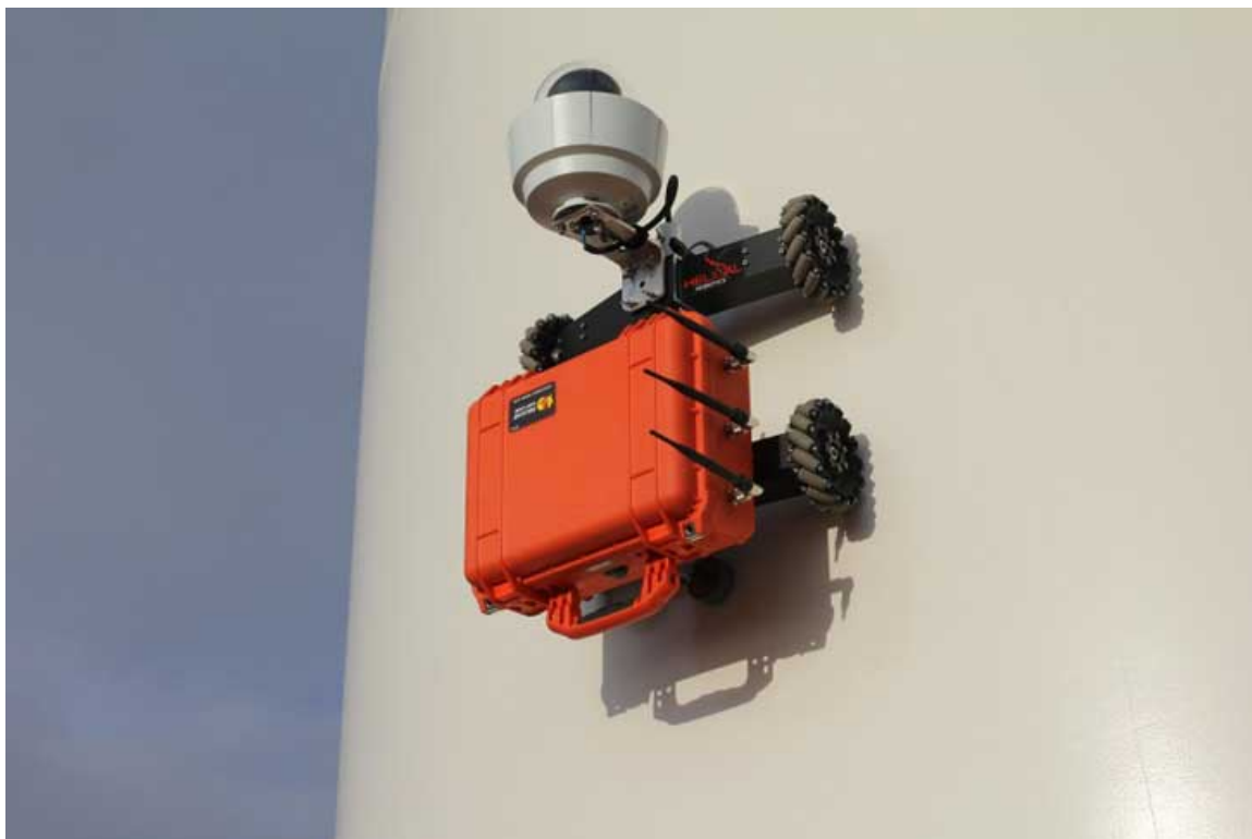
Figure 1.5: Helical robotics robot on wind turbine tower [6]
