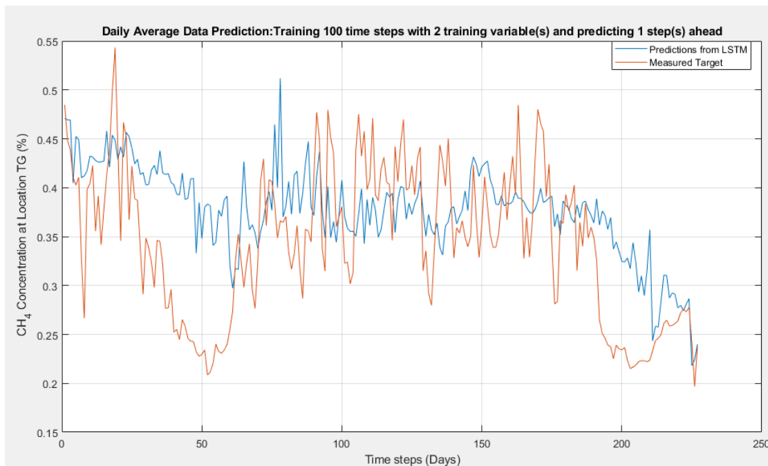
Figure 5-54 LSTM one-step-ahead prediction for the methane concentration at location TG using the unfiltered data and a training window size of one hundred time steps.
