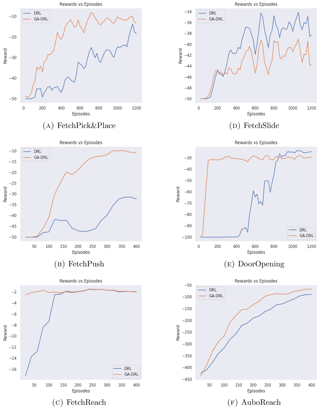
FIGURE 3.13: The DDPG+HER vs. GA+DDPG+HER efficiency evaluation charts are produced when all six hyperparameters are determined using GA (Total reward vs episodes). All graphs are averaged across ten runs. In this figure, DDPG+HER is referred to as DRL.
